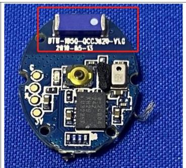
The antenna is Chip antenna. The best case gain of the antenna is 4.97 dBi.
