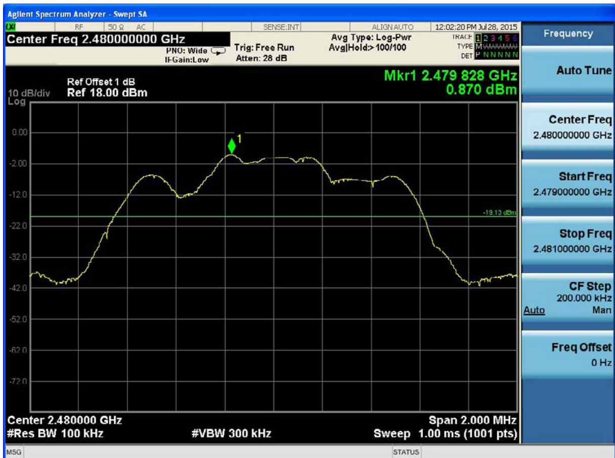
(Plot 4.7.2 C1: Channel 78: 2480MHz @8DPSK)
