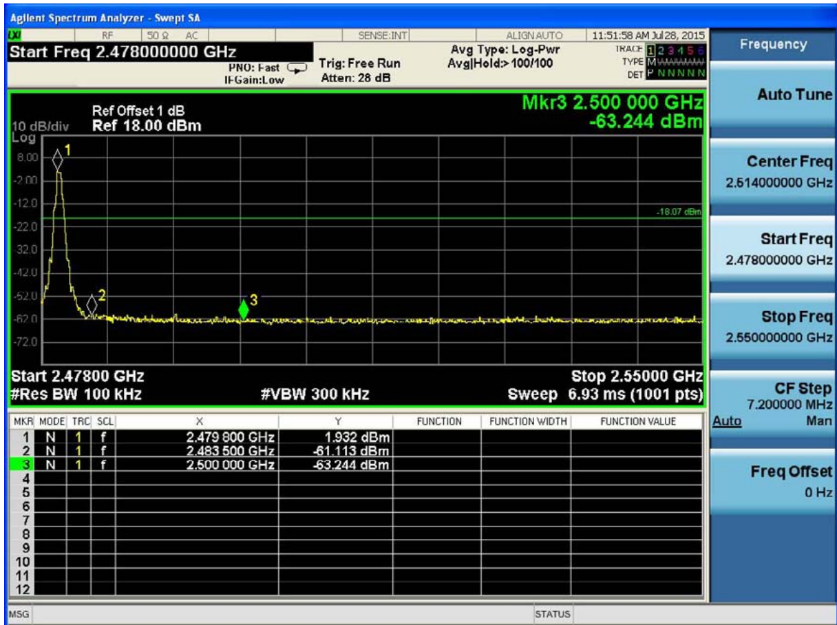
(Plot 4.6.2.1 C: Channel 78: 2480MHz @ GFSK)
