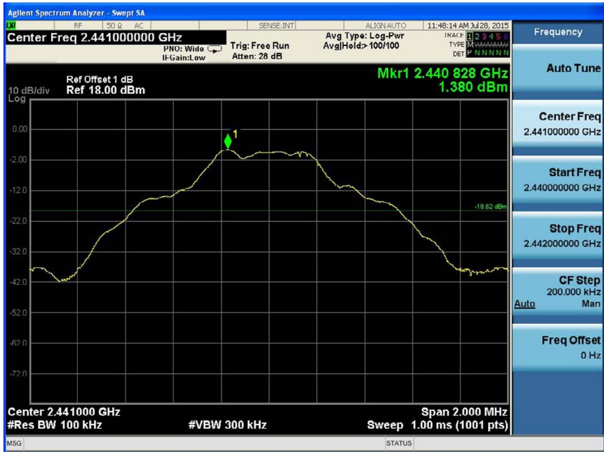
(Plot 4.7.1 B1: Channel 39: 2441MHz @ GFSK)
