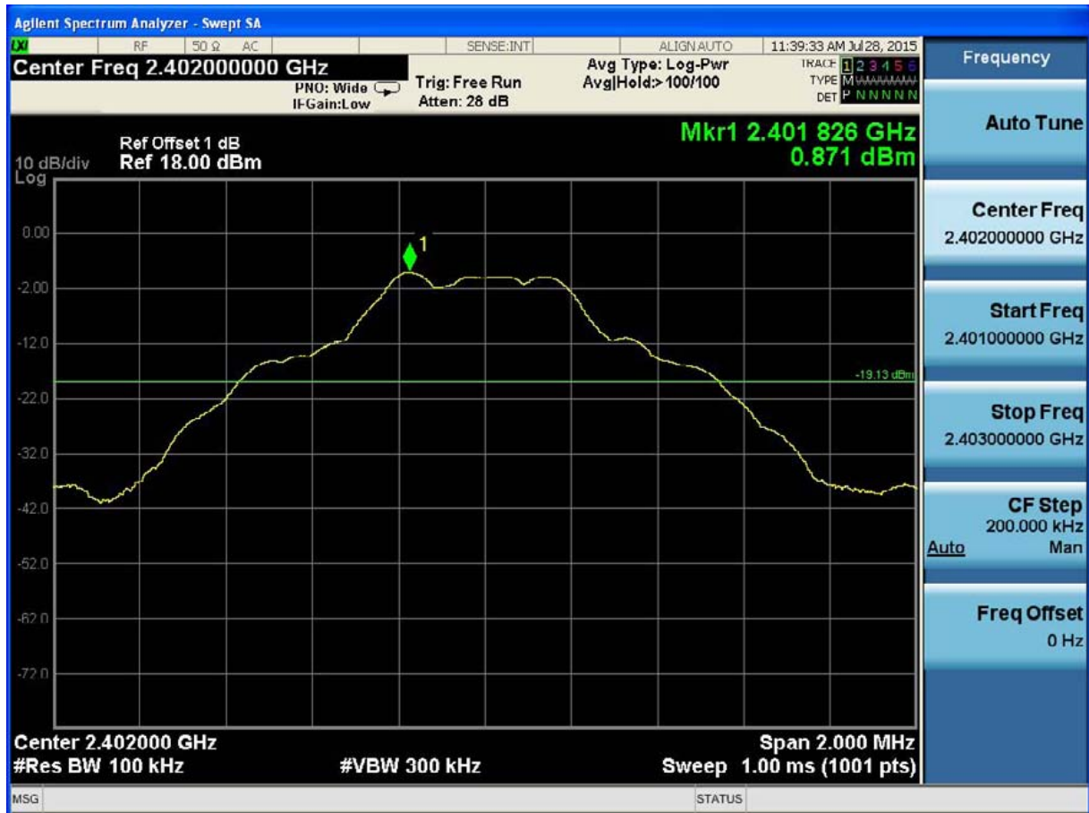
(Plot 4.7.1 A1: Channel 00: 2402MHz @ GFSK)
