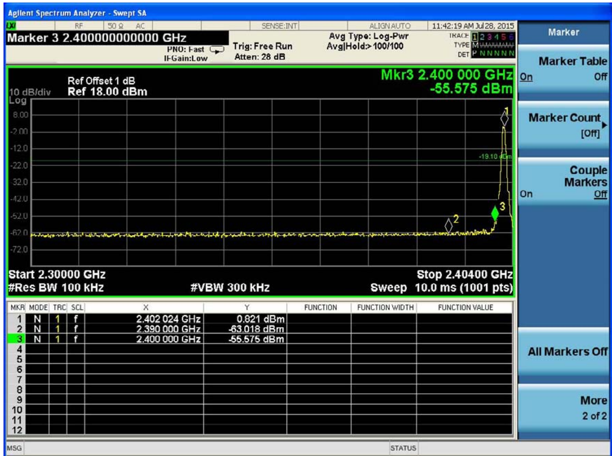
(Plot 4.6.2.1 A: Channel 00: 2402MHz @ GFSK)
