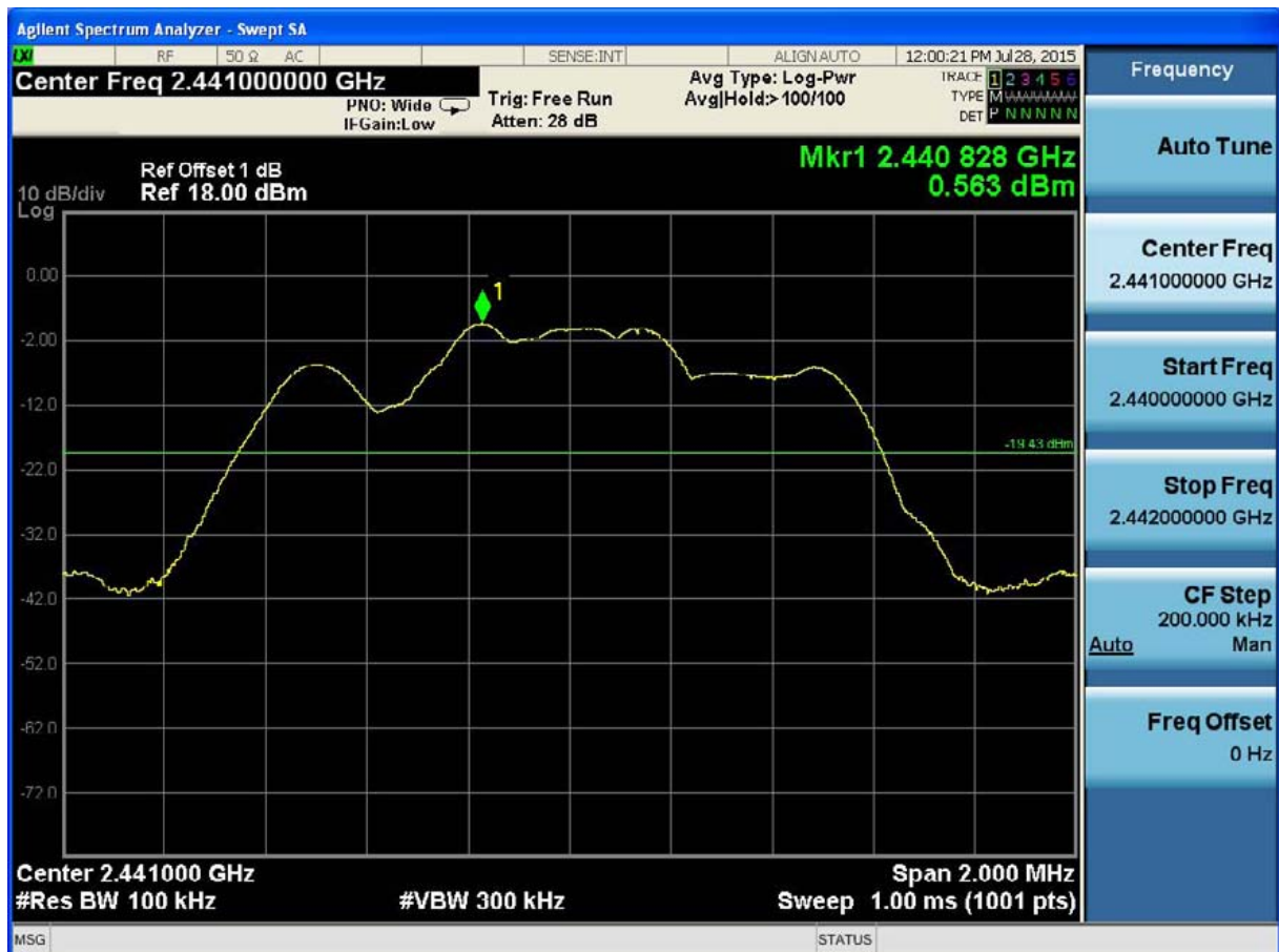
(Plot 4.7.2 B1: Channel 39: 2441MHz @8DPSK)
