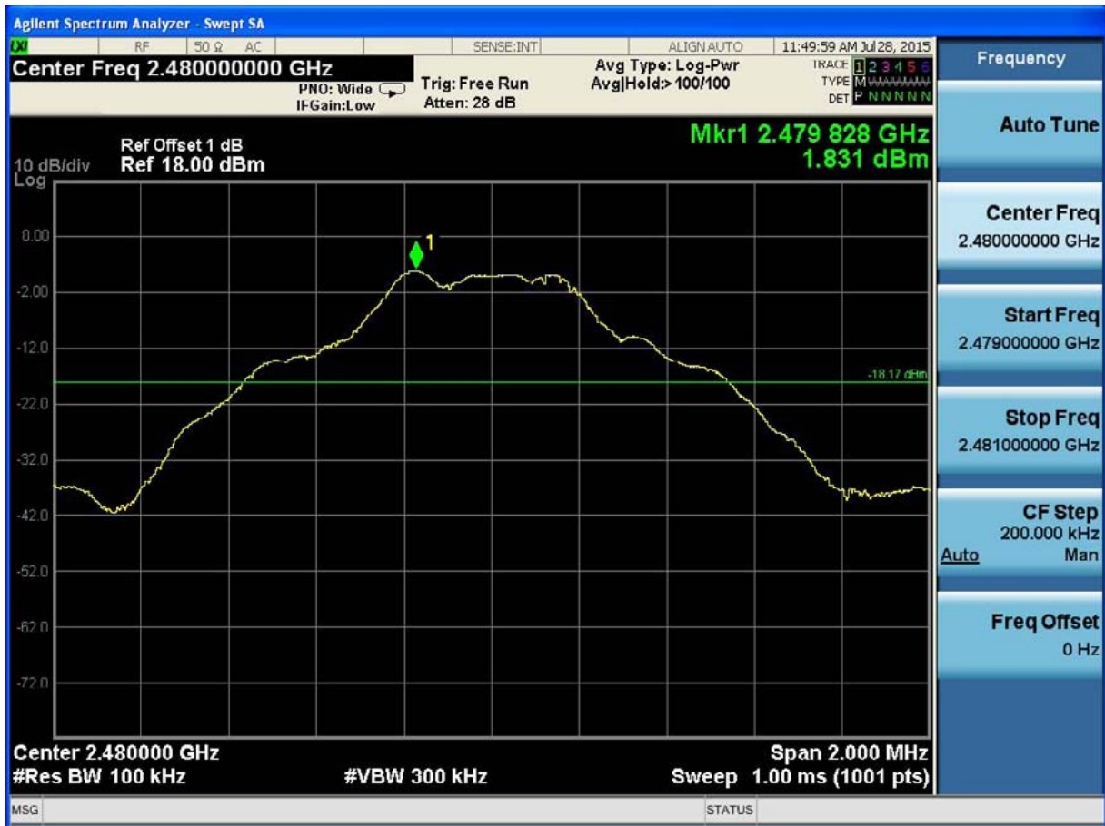
(Plot 4.7.1 C1: Channel 78: 2480MHz @ GFSK)
