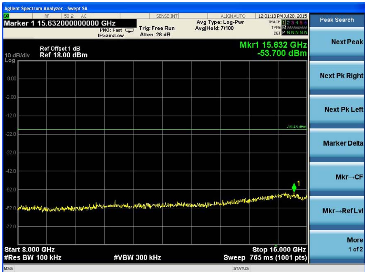
(Plot 4.7.2 B5: Channel 39: 2441MHz @8DPSK)
