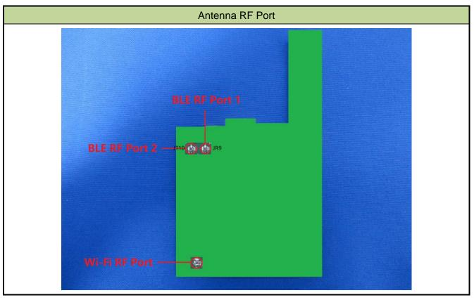
Note: The Bluetooth module has two RF ports (JR9 and JR10), only the JR9 port can transmit, the JR10 is reserved that can't transmit by the manufacturer.
