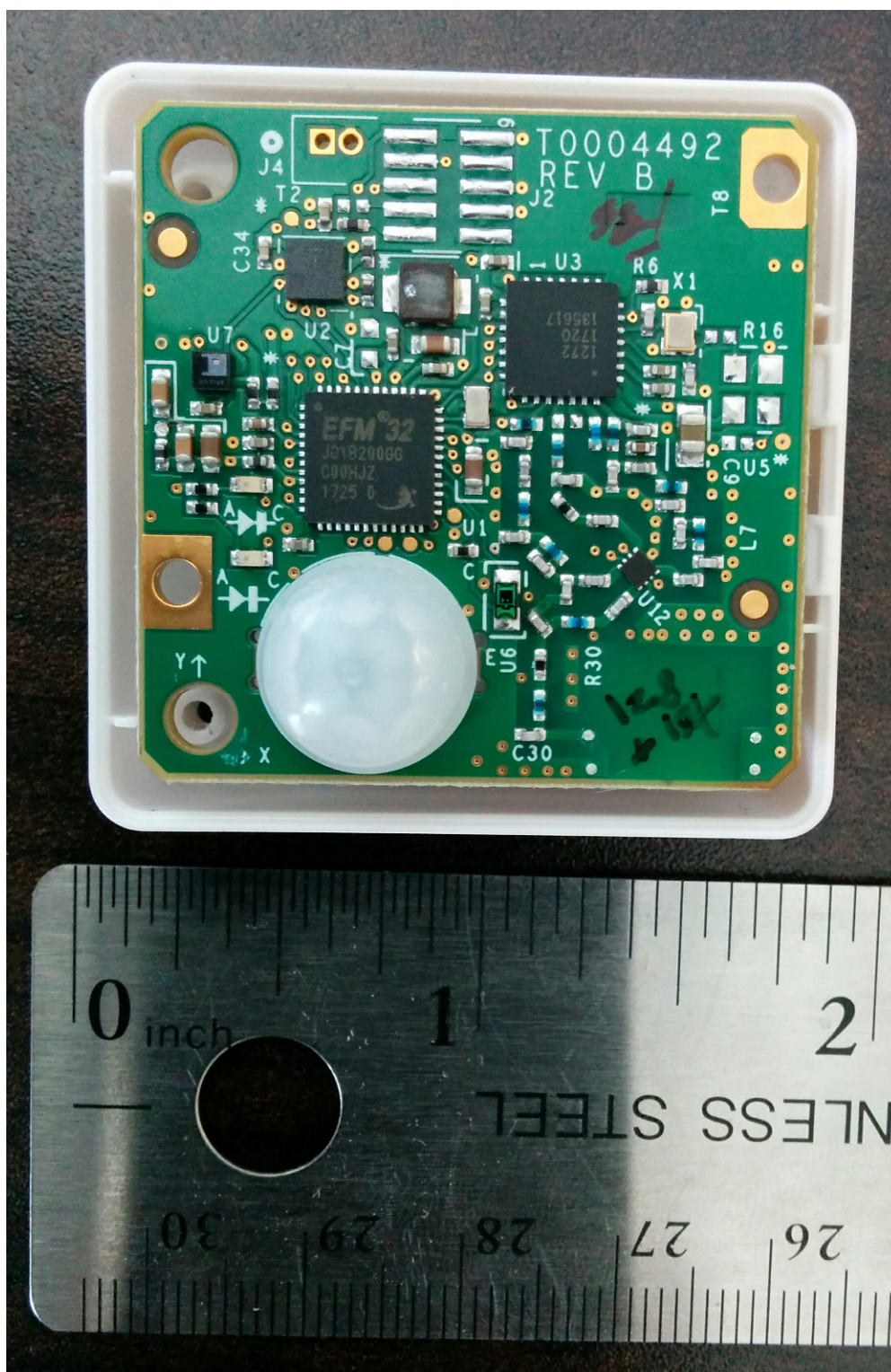
T0004885 in Enclosure (PIR Sensor)
