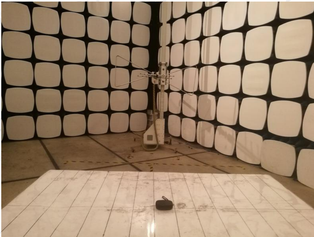
FCC RADIATED EMISSION TEST SETUP
