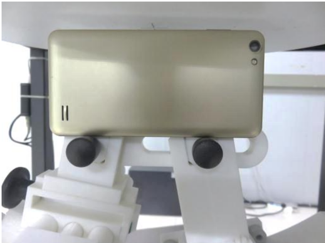
10mm body-worn Left Side Setup Photo(hotspot)
