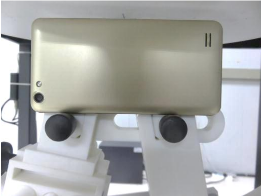
10mm body-worn Right Side Setup Photo(hotspot)
