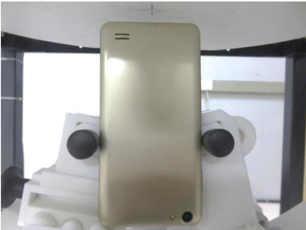
10mm body-worn Bottom Side Setup Photo(hotspot)
