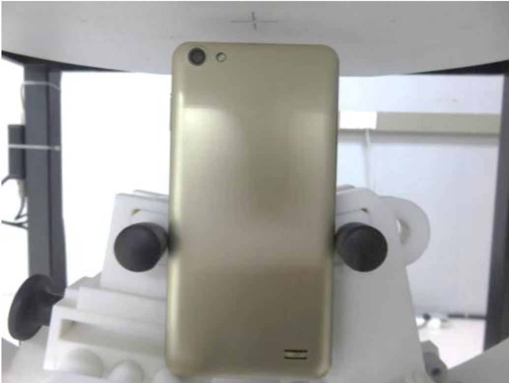
10mm body-worn Top Side Setup Photo(hotspot)
