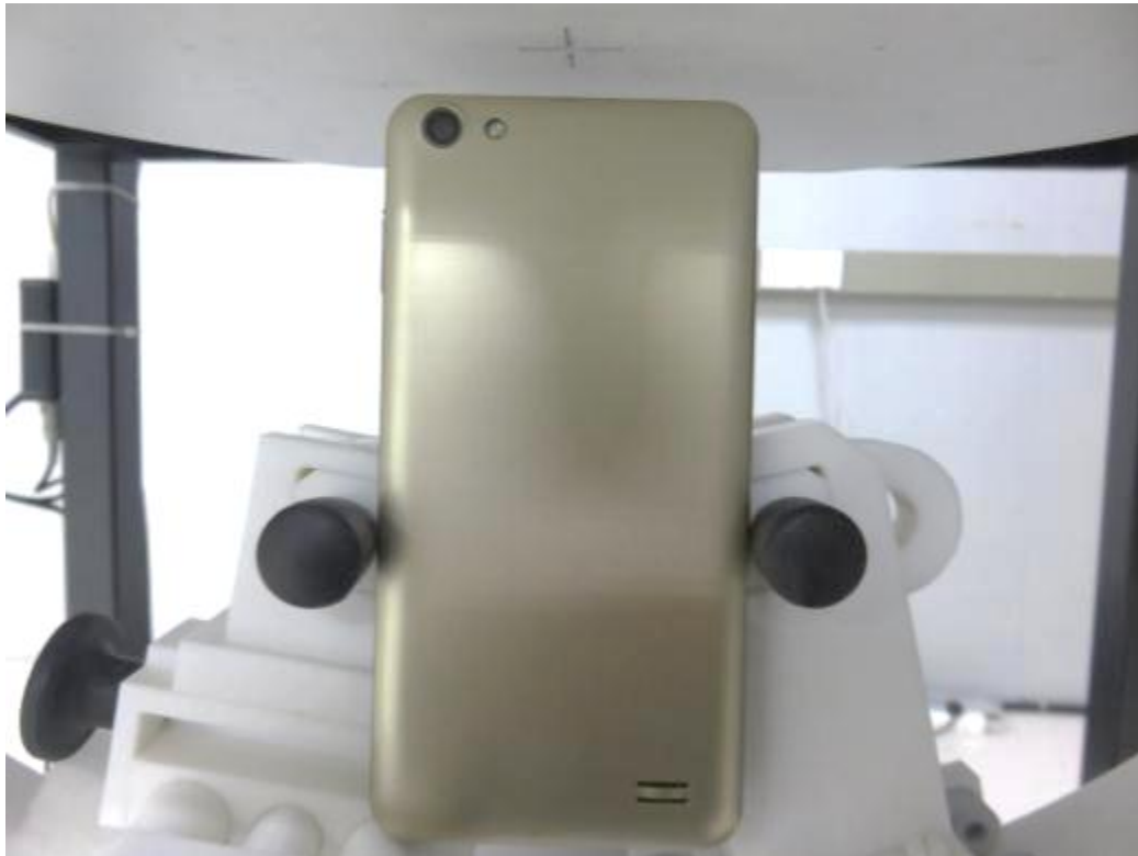
10mm body-worn Top Side Setup Photo(hotspot)
