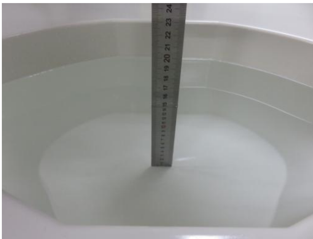
Photograph of the depth in the Body Phantom (5000MHz, 16.3cm depth)
