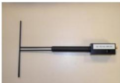
Figure 1 – Satimo COMOSAR Validation Dipole
