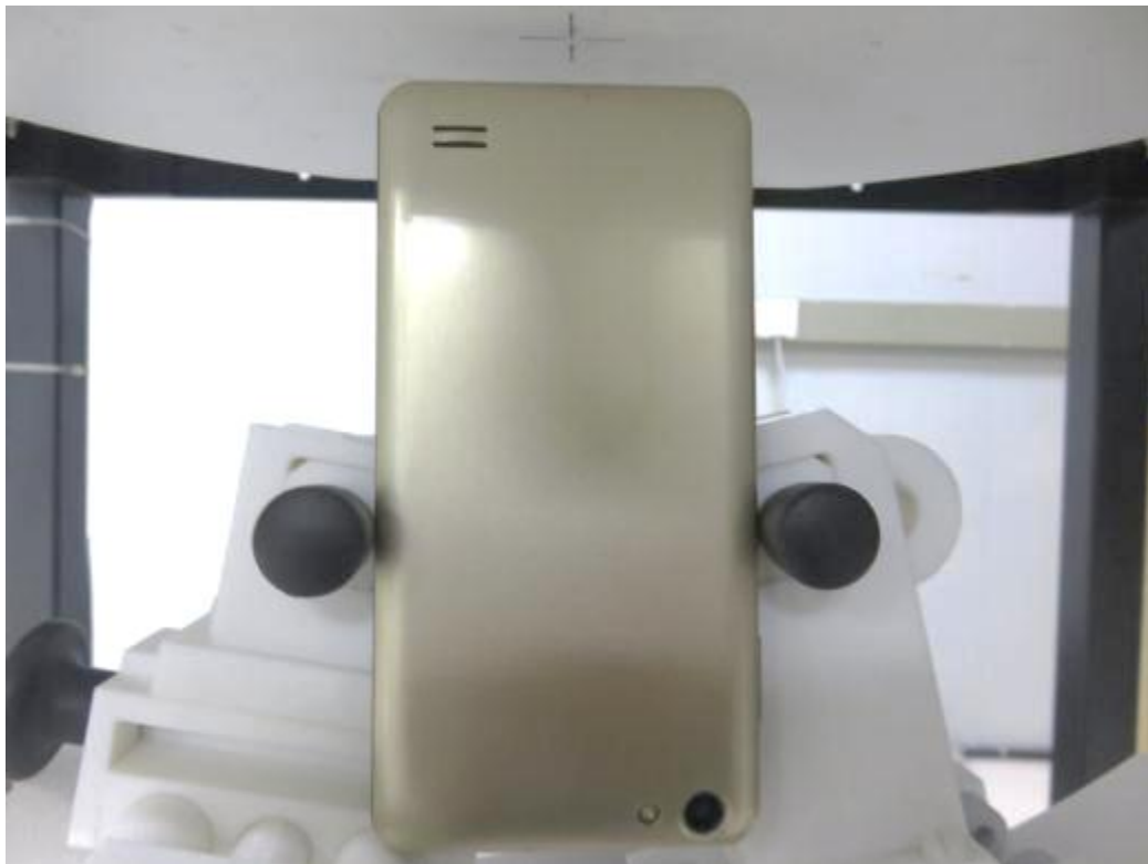
10mm body-worn Bottom Side Setup Photo(hotspot)
