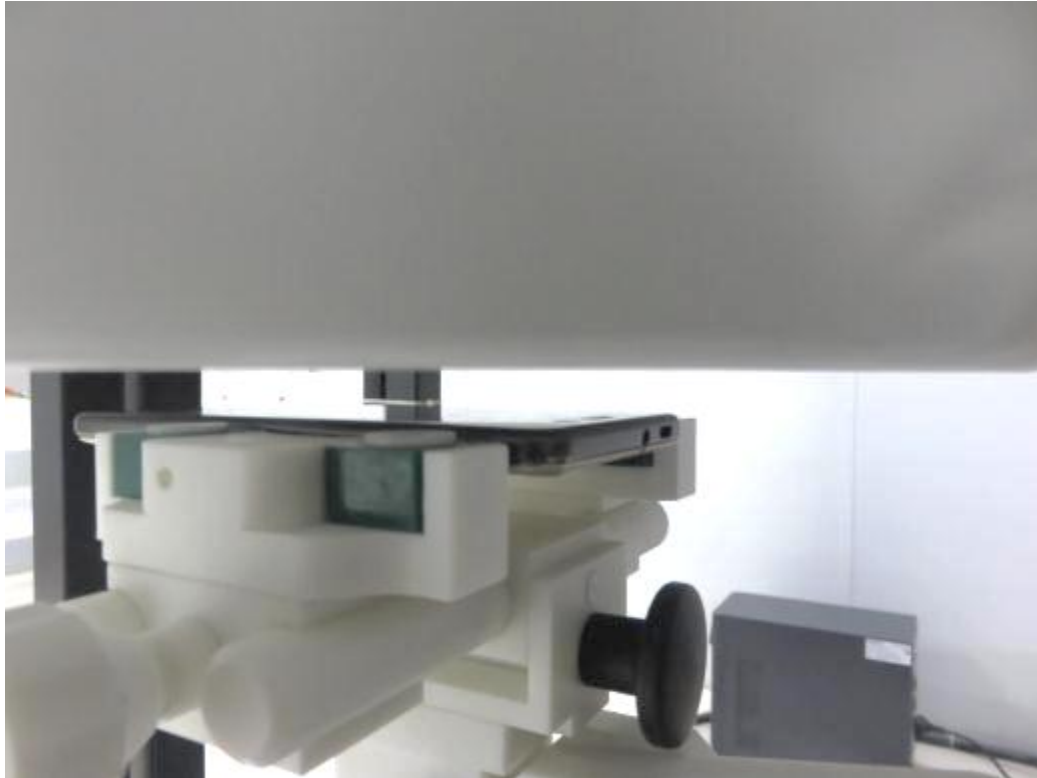
10mm body-worn Back Side Setup Photo(hotspot)
