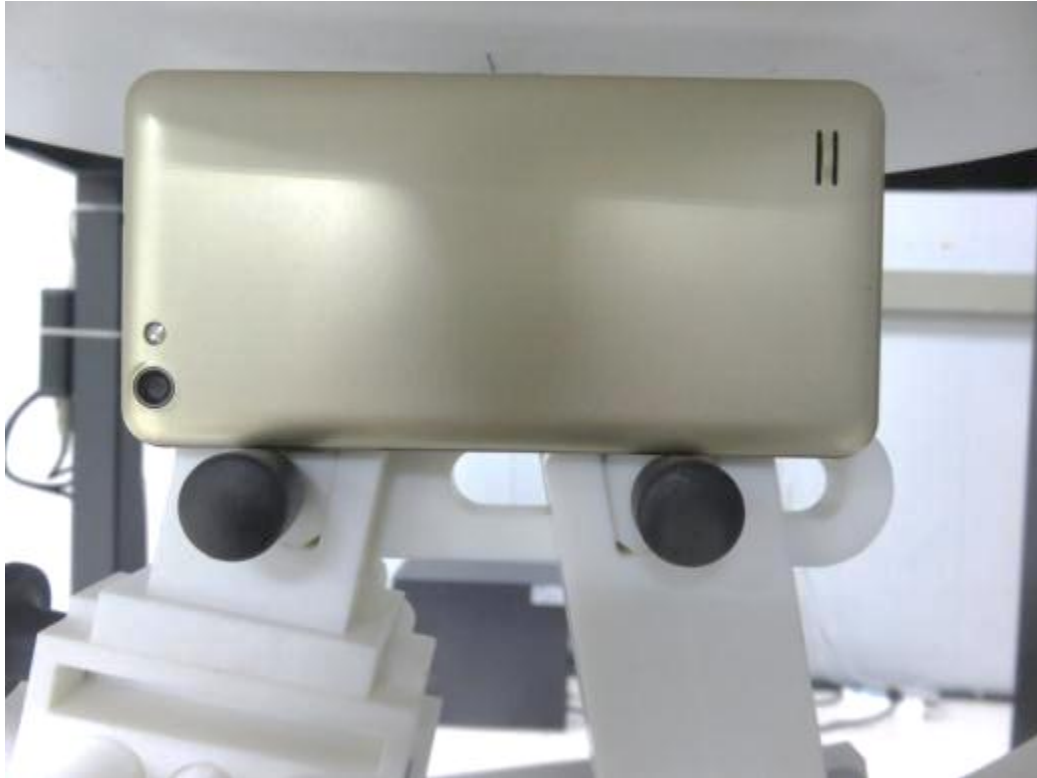
10mm body-worn Right Side Setup Photo(hotspot)
