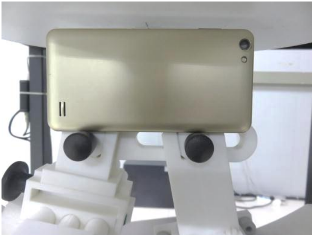
10mm body-worn Left Side Setup Photo(hotspot)
