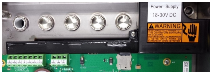
Figure 2-5: DC Power input Connector with Cover
