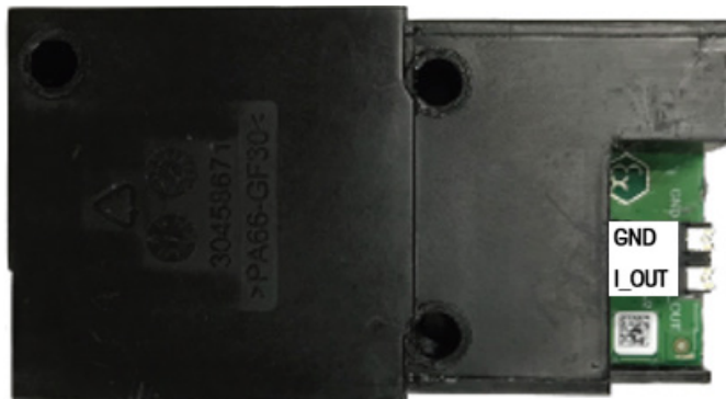
Figure 2-12: Intrinsically Safe Analog Output Option Board
