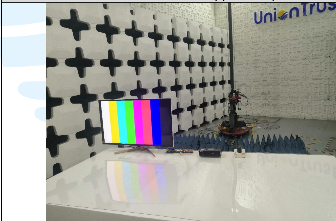
Radiated emission Test Setup (Above 1 GHz)
