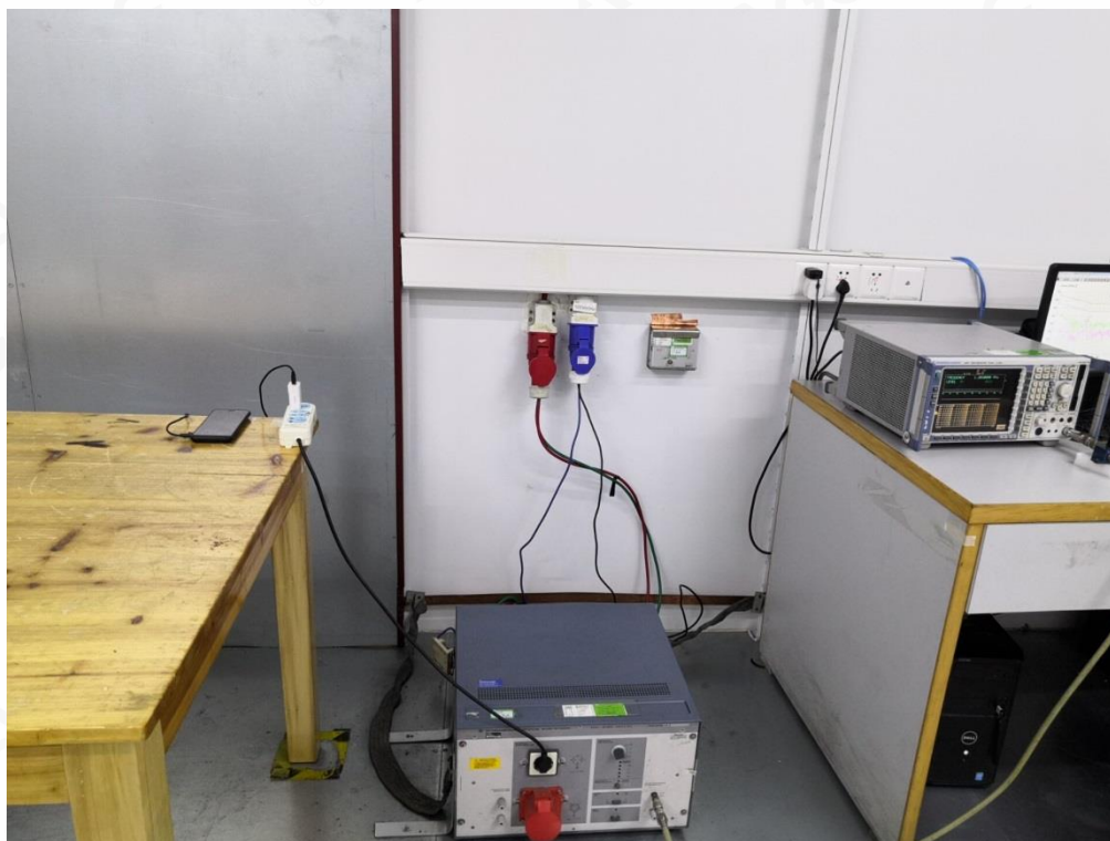
RADIATED EMISSION TEST SETUP BELOW 1GHZ
