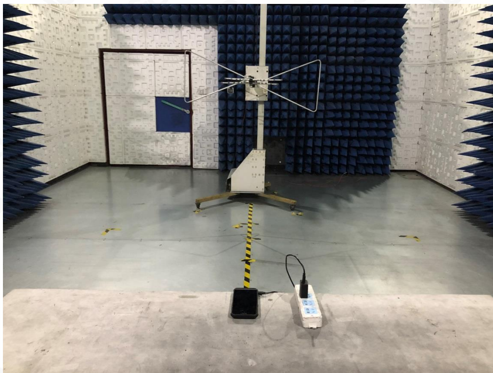
RADIATED EMISSION TEST SETUP BELOW 1GHZ
