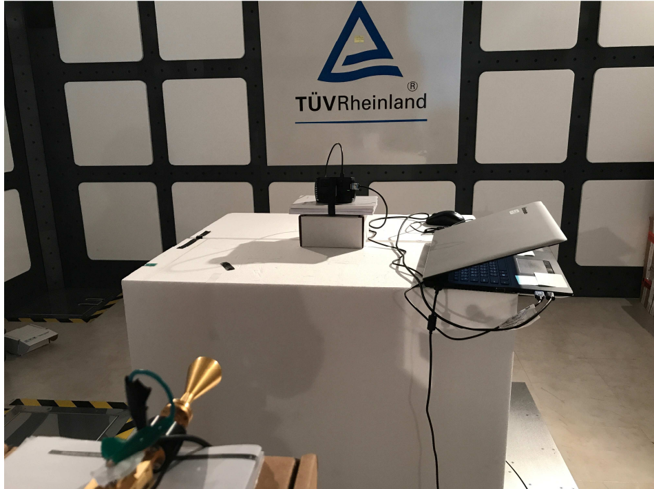
Photograph 4: Set-up for Spurious Emissions (Above 40GHz)
