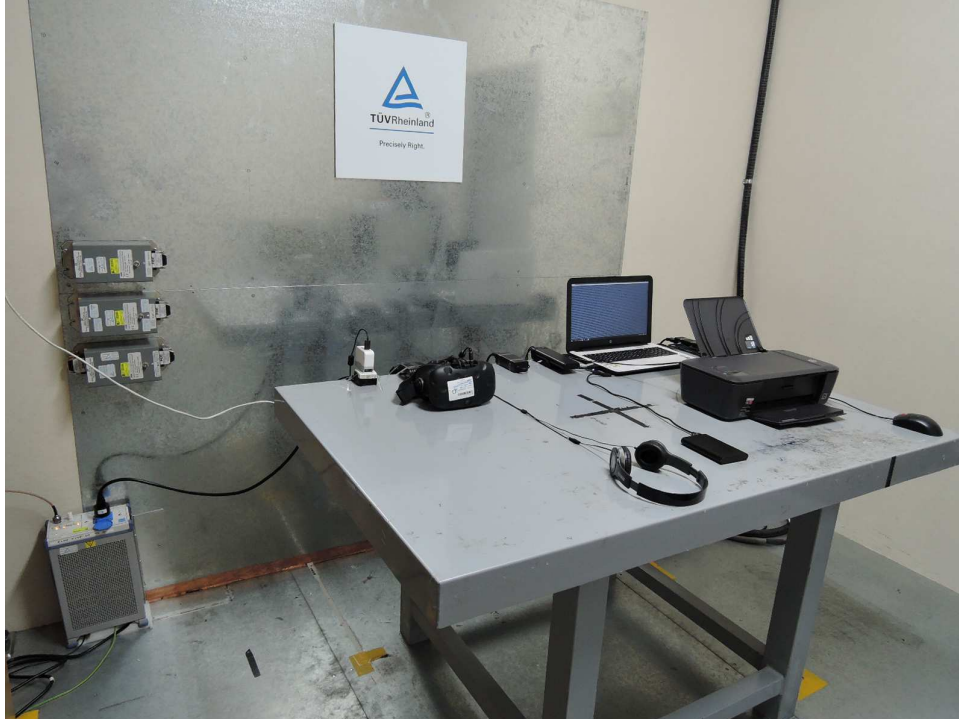
Photograph 6: Set-up for for Mains Conducted testing Front
