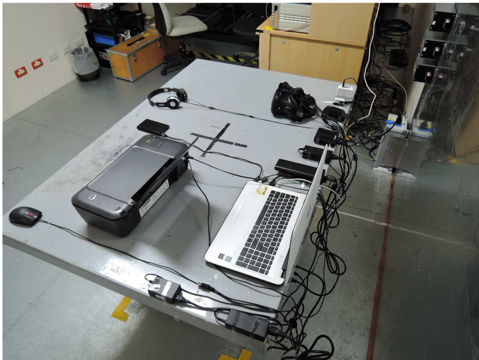
Photograph 5: Set-up for for Mains Conducted testing Back
