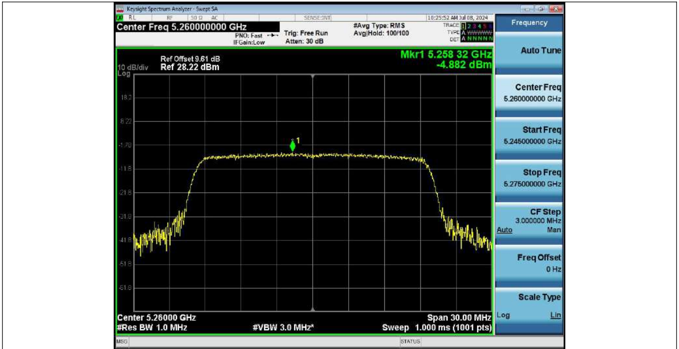
Power Spectral Density_NVNT_ANT1_802_11ax(HE20)_5300
