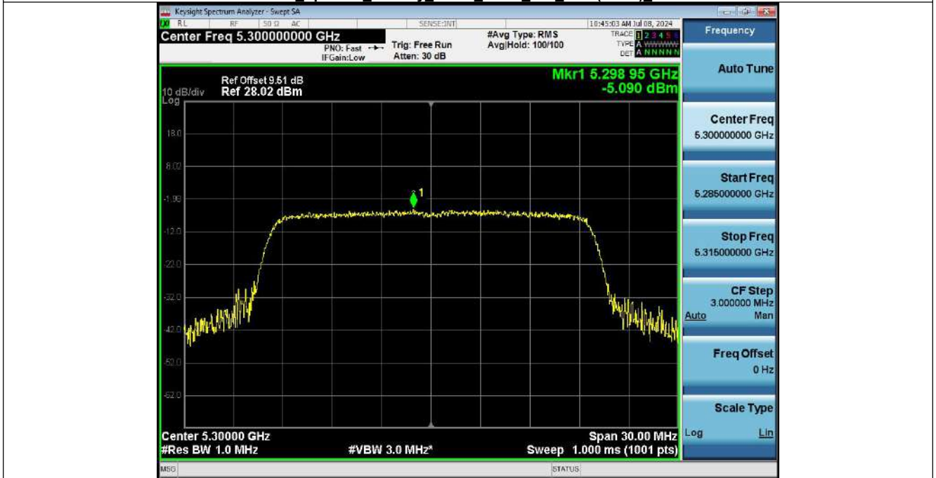
Power Spectral Density_NVNT_ANT1_802_11ax(HE20)_5300
