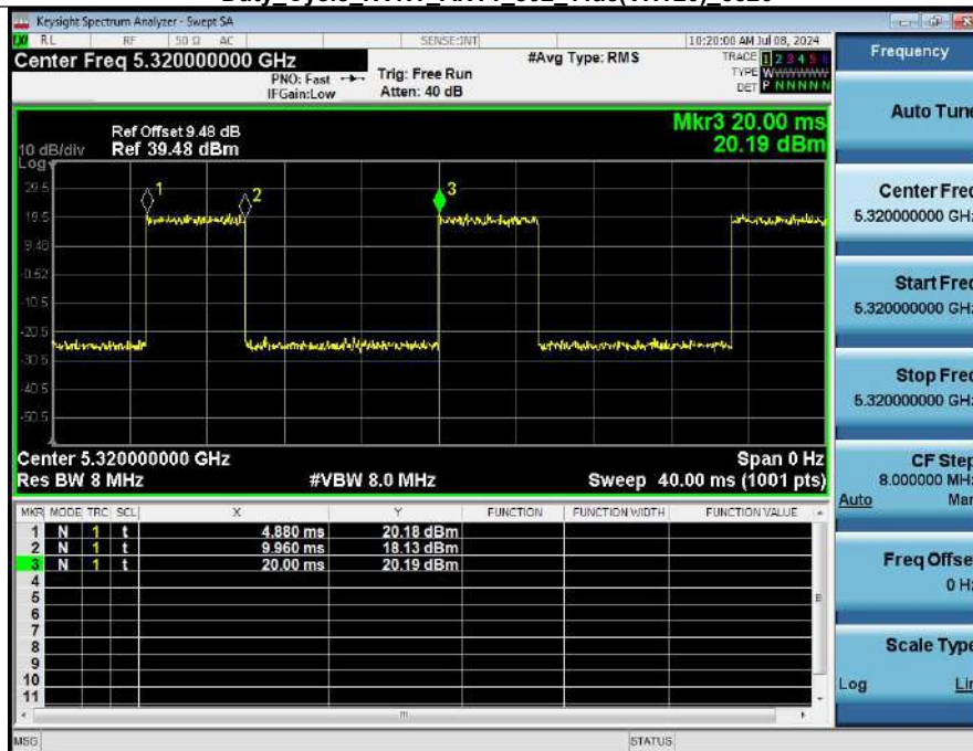
Duty Cycle NVNT ANT1 802_11ac(VHT20) 5320
