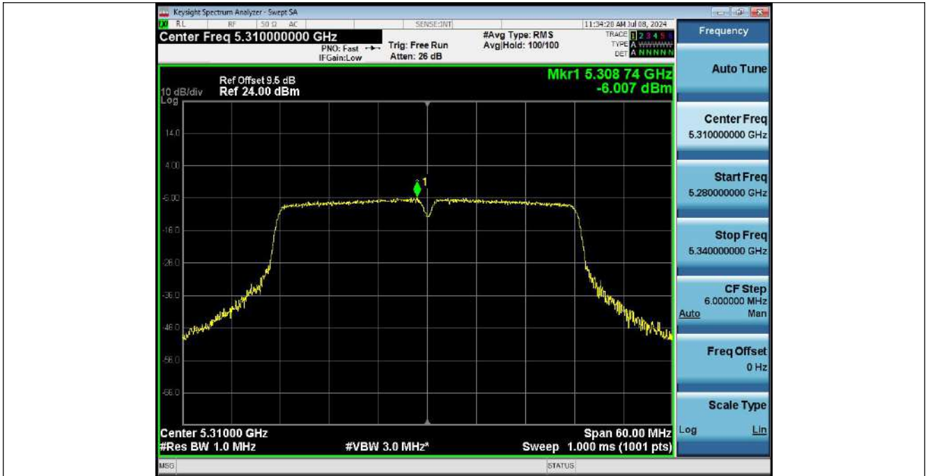
Power Spectral Density_NVNT_ANT1_802_11ax(HE40)_5270
