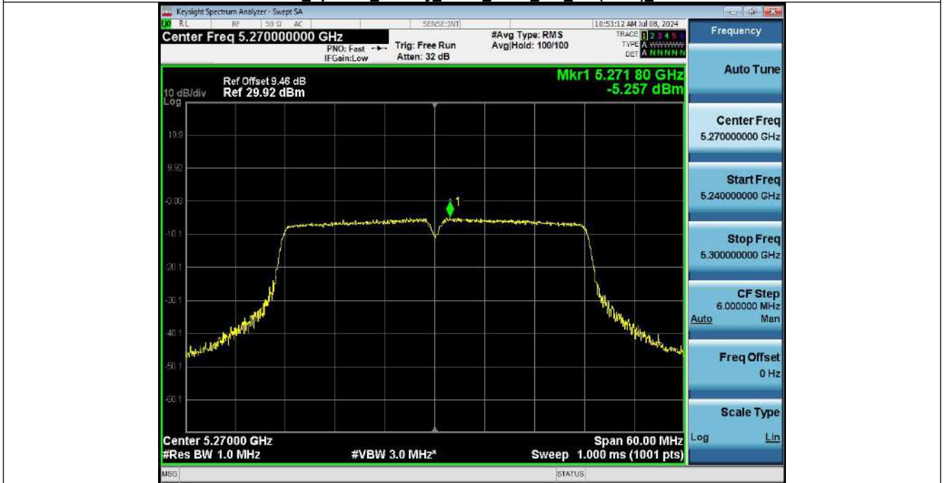
Power Spectral Density NVNT ANT1 802_11n(HT40)_5270
