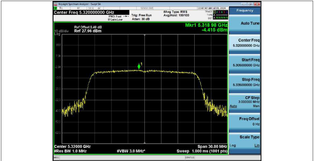
Power Spectral Density NVNT ANT1 802_11n(HT40)_5270
