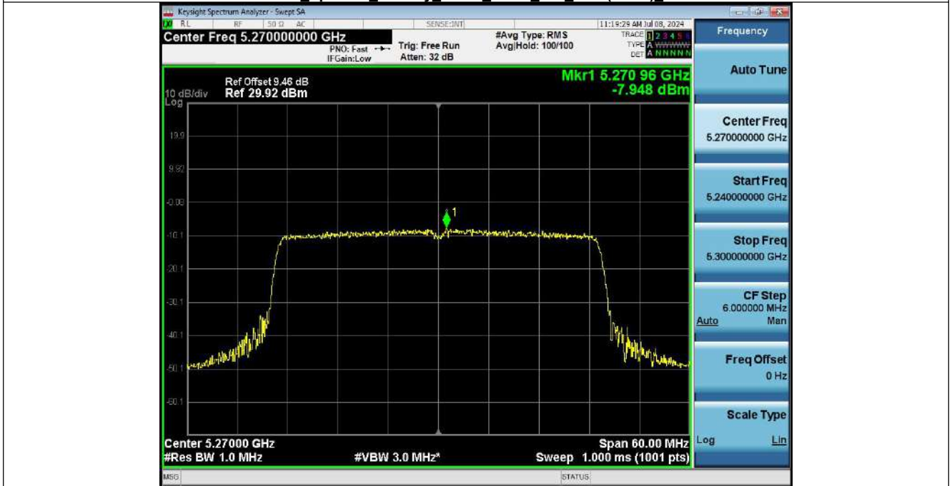
Power Spectral Density_NVNT_ANT1_802_11ax(HE40)_5270
