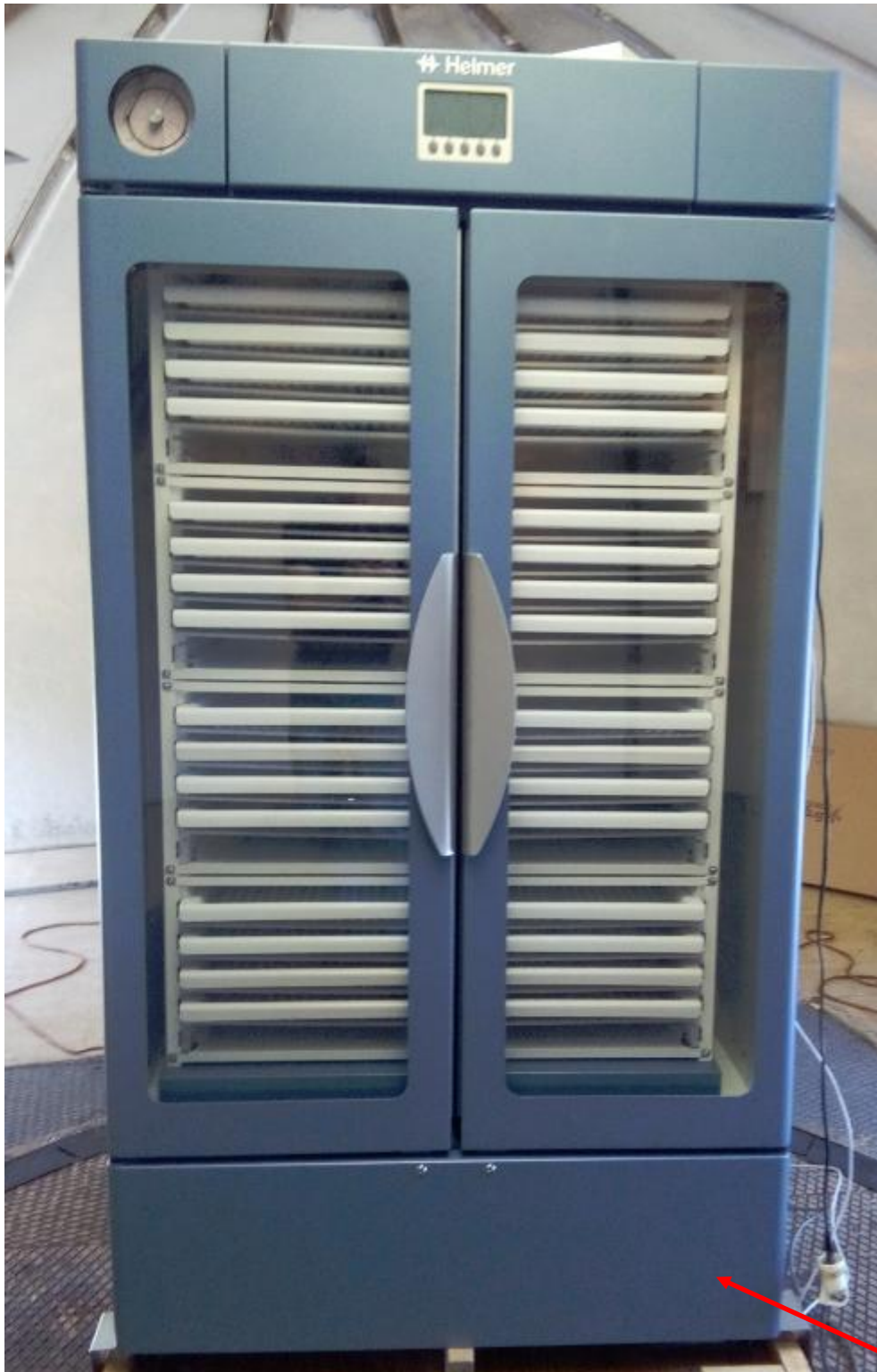
In this product, the agitator and incubator functions are in a single ELMER product (PC4200).
