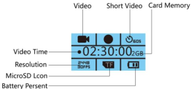
Click "OK" to start recording, you can see the recording time and video mode on the LCD screen.
