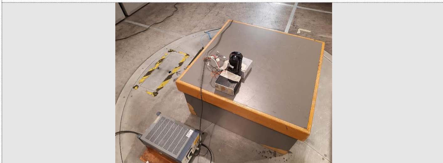
PHOTO N° 3 - CONDUCTED EMISSION TEST SETUP
