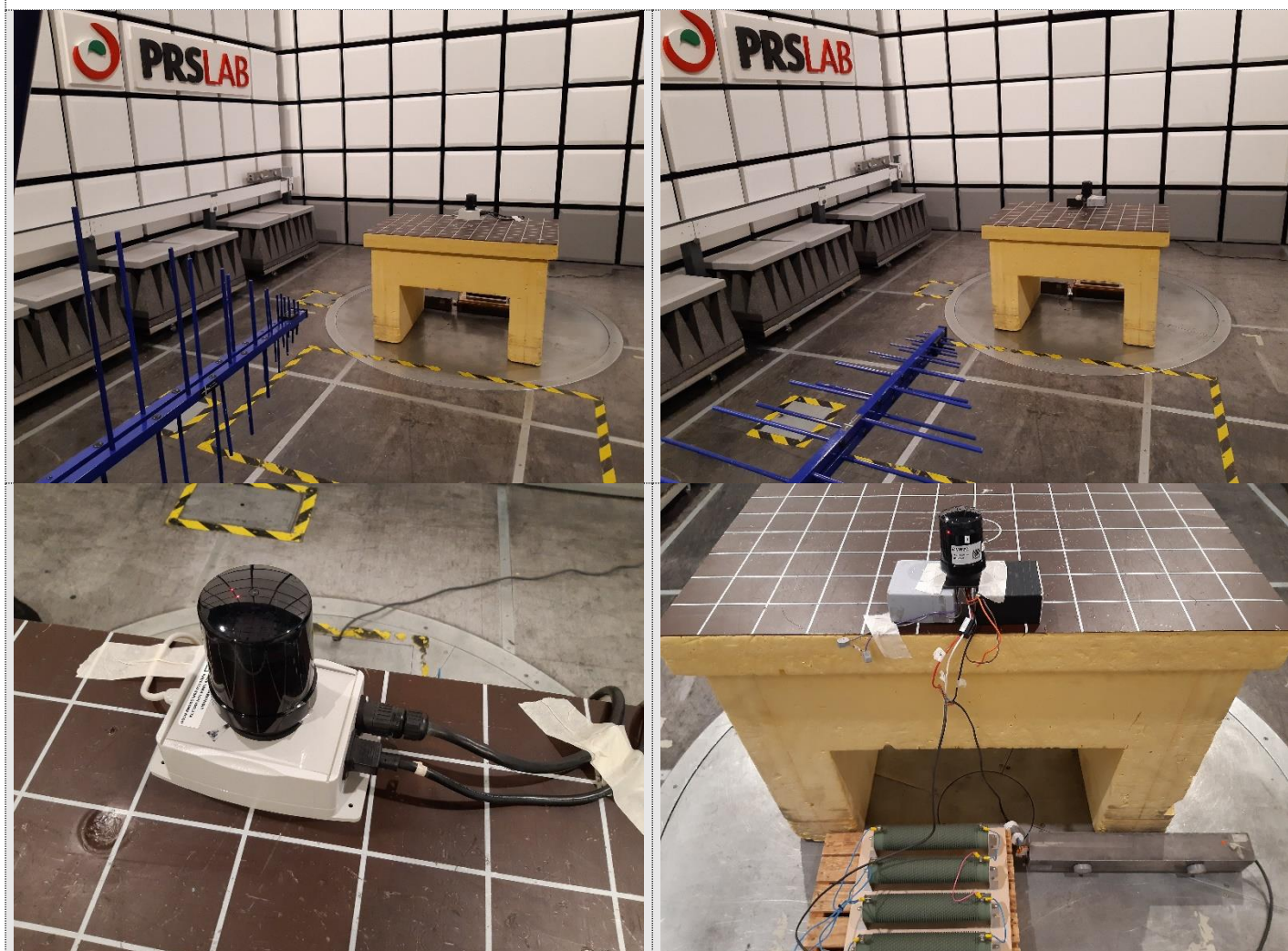
PHOTO N° 2 - RADIATED EMISSION TEST SETUP
