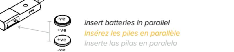
insert batteries in parallel
