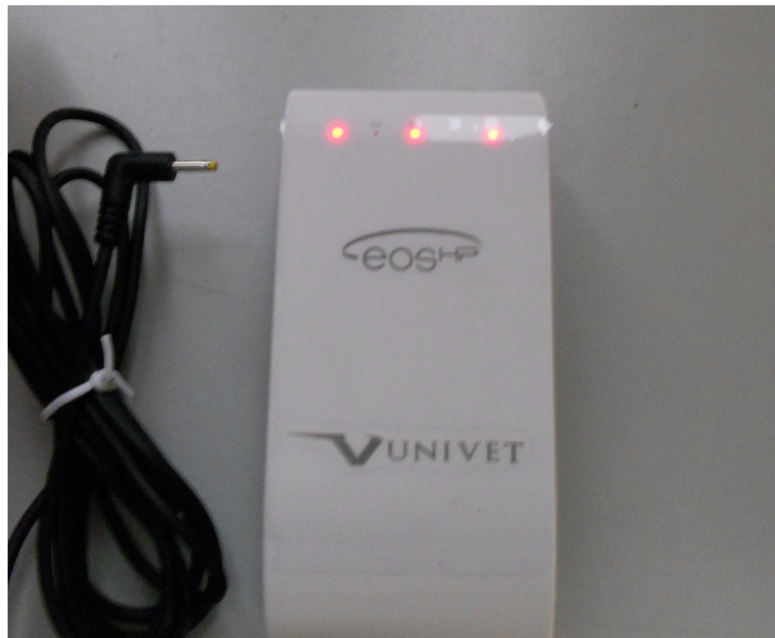
LED SIGNALLING RED LED = HEADLAMP UNCONNECTED OR FAULT
