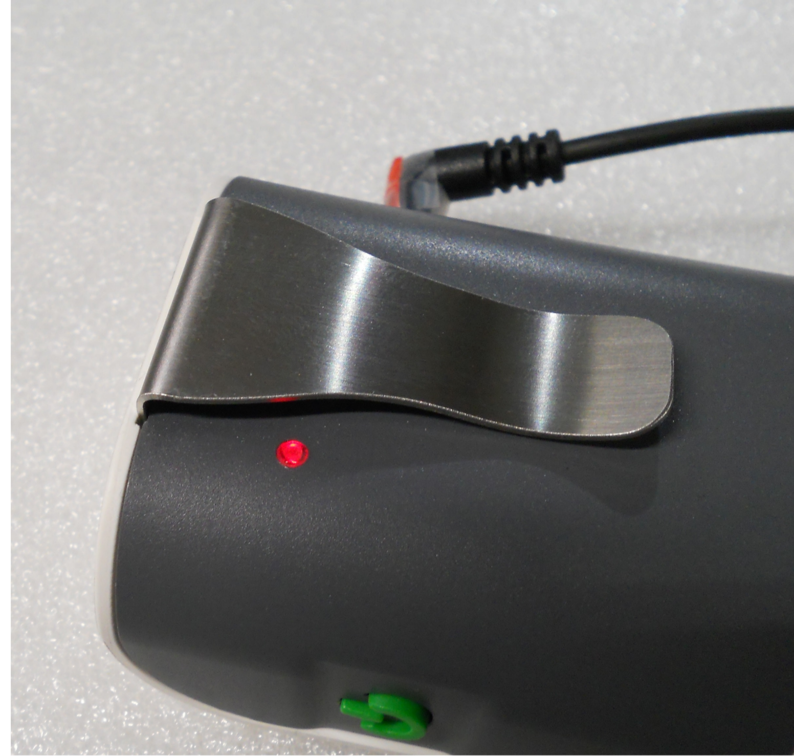
LED SIGNALLING BACKSIDE LED = DEVICE IN CHARGE
