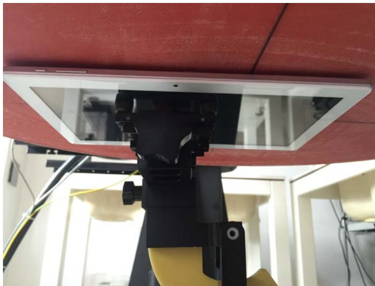
Test Position 1 - Body-worn, the rear side of the EUT towards phantom (The distance was 0mm)
