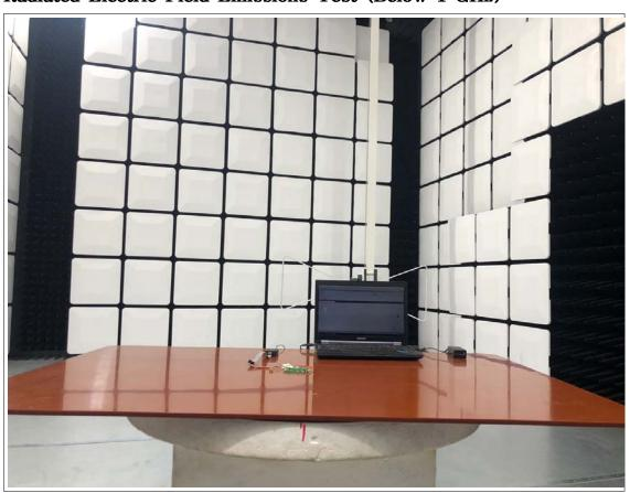
Radiated Electric Field Emissions Test (Above 1GHz)
