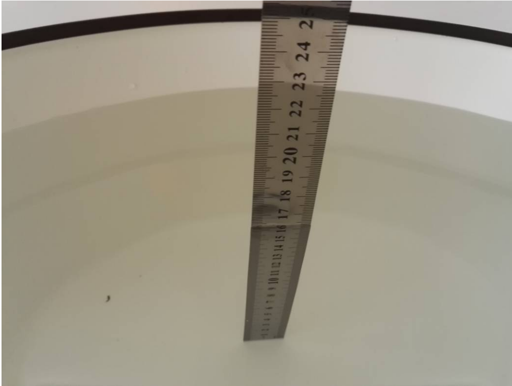
Liquid depth \geq 15\text{cm}
