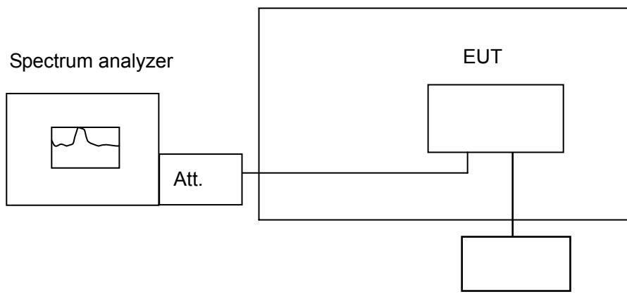
**Remark:** Measurement setup for testing on Antenna connector
