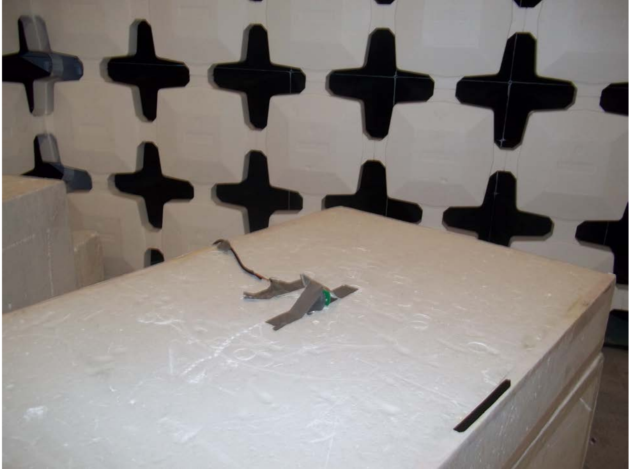
Figure 1. Radiated Emissions Test Setup, BT Radio
