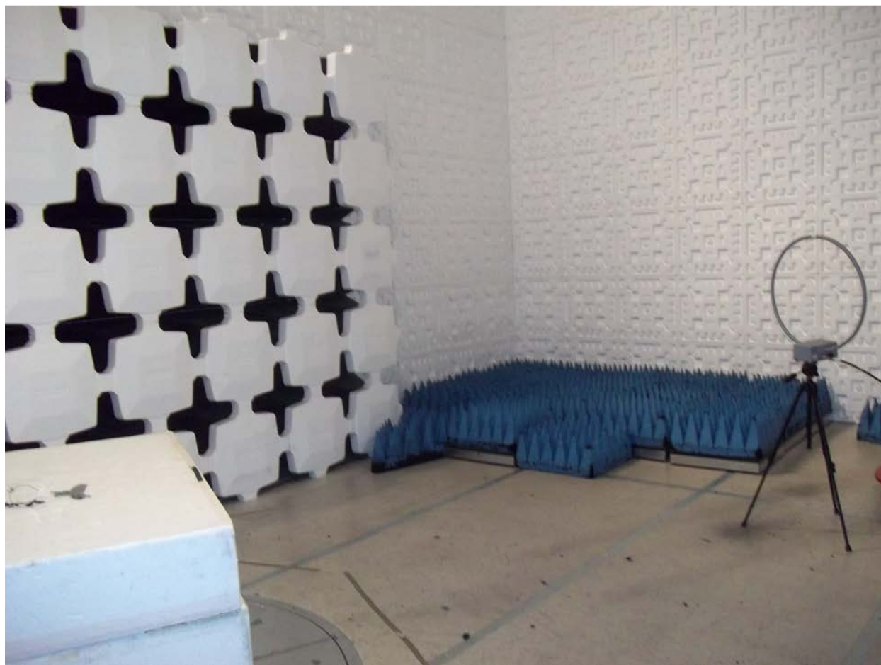
Figure 3. Radiated Emissions Test Setup (9 kHz - 30 MHz)
