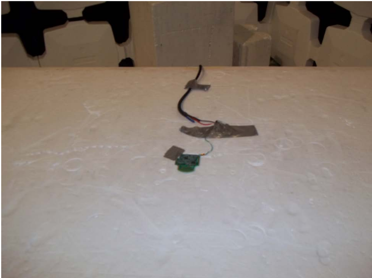
Figure 2. Radiated Emissions Test Setup, UHF (433-435 MHz) Radio
