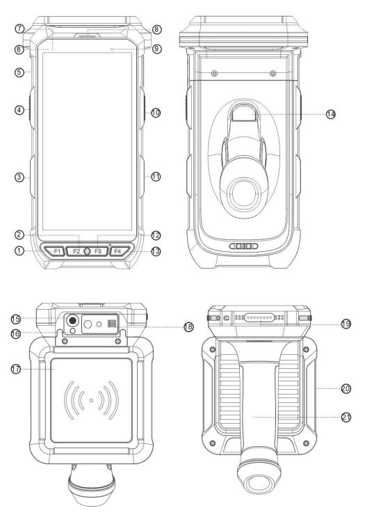
①F1 ②F2 ③Volume ④ Reserved Button ⑤ USB port ⑥ Blue Led Indicator ⑦ Red LED indicator ⑧ Receiver ⑨ Front Camera ⑩ Reserved Button ⑪ Power Button ⑪ F3 ⑪ F4 ⑭ Pistol Grip Button ⑤ Rear Camera ⑯ Flashlight ⑰ UHF Shield ⑱ Barcode Scan Window ⑲ Cradle Pogo Pin Connector ㉑ UHF Shield Metal Housing ㉑ Pistol Grip
