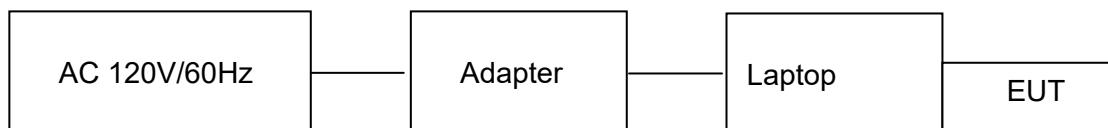
Operation of EUT during Radiated testing
