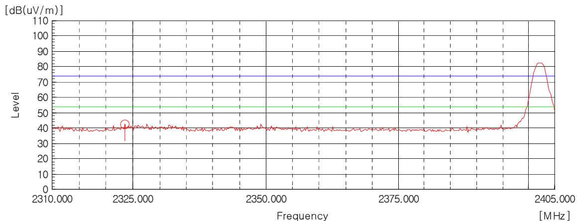
AV Detector: RBW: 1 MHz, VBW: 10 Hz (2 310 MHz - 2 390 MHz), Worst case (Low, Horizontal)
