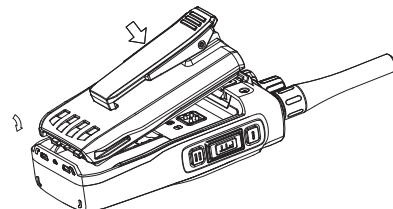
To install the battery fit in the battery to the battery compartment from the bottom of the battery. Press the top part of the battery towards the IP smart terminal until a click is heard. The battery is locked in place.
