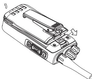
To remove the battery – power off the terminal, push the battery lock upwards subsequently pull the top part of the battery away from the IP smart terminal. Lift up the whole battery.
