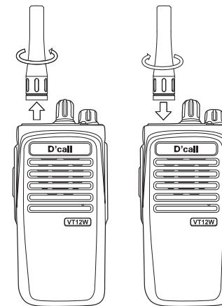
Align the treaded end of the antenna with the IP smart terminal's antenna socket then turn the antenna clockwise to fasten it.
