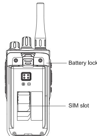
Insert the SIM Card into the SIM slot as shown in the picture.
