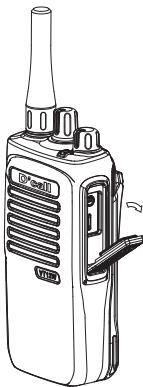
Lift the audio accessory dust cover and insert the earphone or USB cable plug into the relevant socket.
