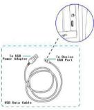
Connect the IP smart terminal and power adapter using the USB Data Cable.
