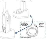
Connect the Desktop Charger and the Power Adapter using the USB Data Cable.
