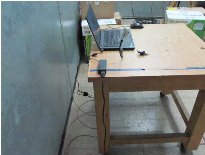
Photo 6. Conducted emissions test setup.
