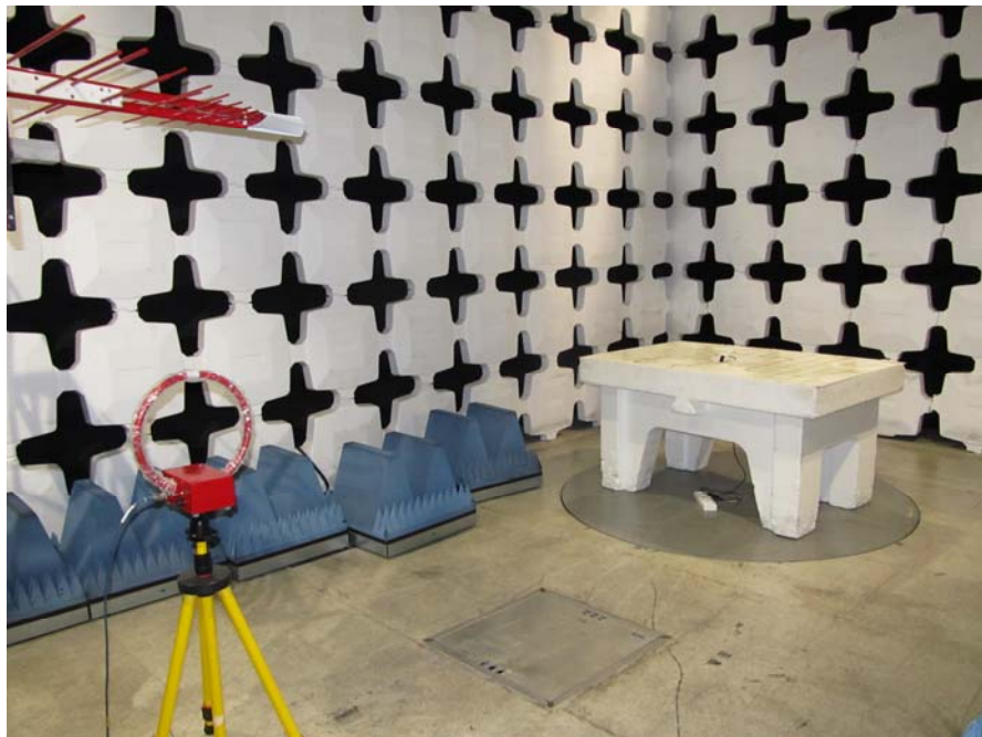
Photo 1.. Radiated emissions test setup with Loop and Biconilog antenna.
