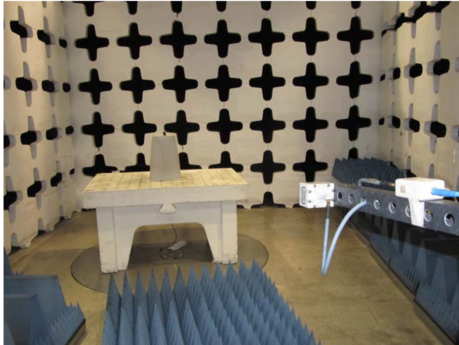
Photo 3. Radiated emissions test setup with Horn antenna in 18-25GHz.
