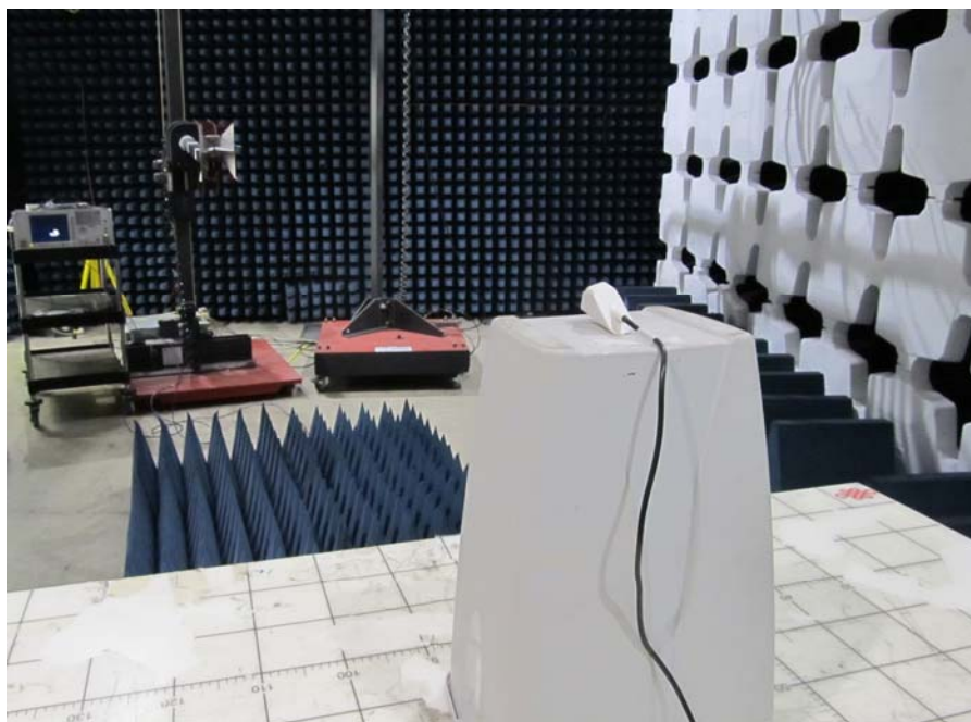
Photo 2. Radiated emissions test setup with Horn antenna in 1-18GHz.
