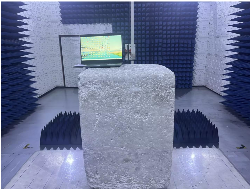
RADIATED EMISSION TEST SETUP ABOVE 1GHz
