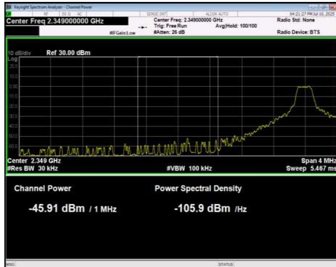
Band40(2350-2360) QPSK BW=10MHz Channel=39200 RB Size=1 Position=#0 Normal
