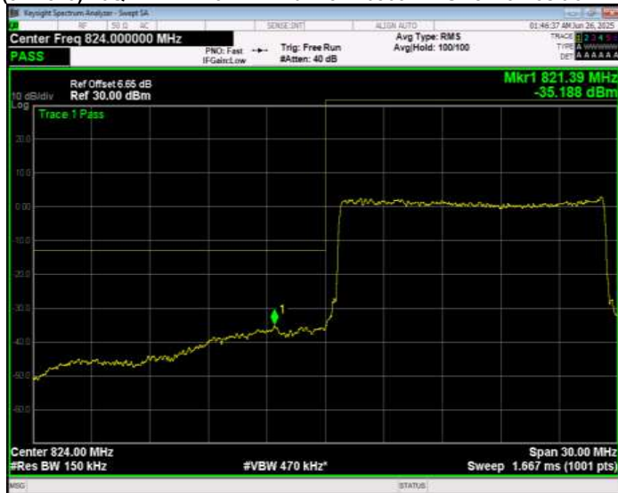
Band26(824-849) 16QAM BW=15MHz Channel=26965 RB Size=1 Position=#0 Normal
