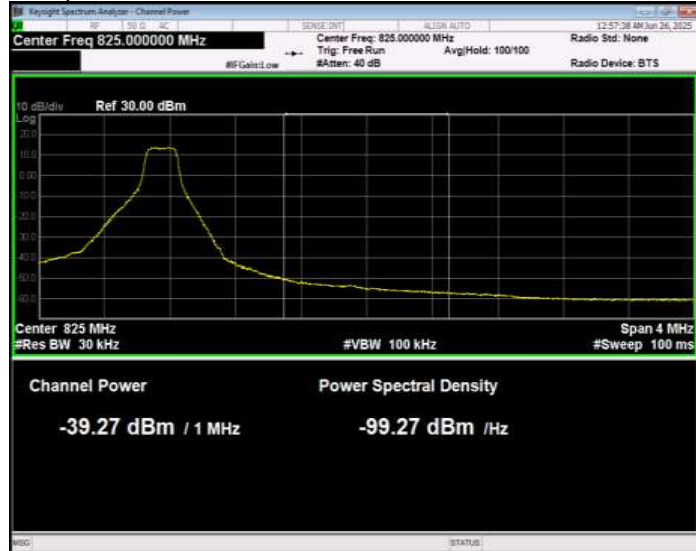
Band26(814-824) 16QAM BW=1.4MHz Channel=26783 RB Size=1 Position=#Max Normal
