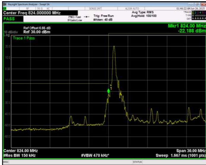
Band26(824-849) QPSK BW=15MHz Channel=26865 RB Size=1 Position=#Max Normal
