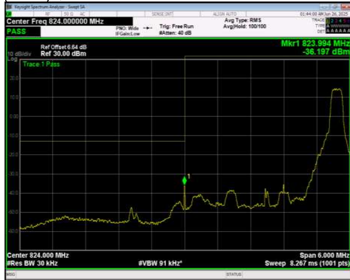
Band26(824-849) QPSK BW=3MHz Channel=26805 RB Size=15 Position=#0 Normal
