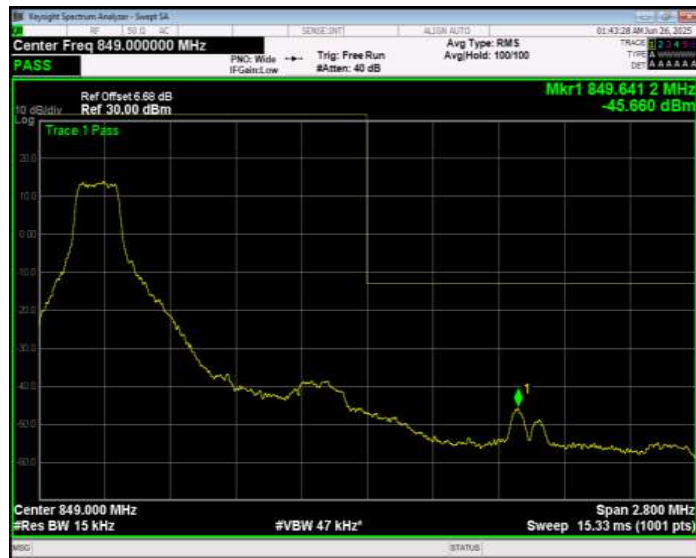
Band26(824-849) QPSK BW=1.4MHz Channel=27033 RB Size=1 Position=#Max Normal
