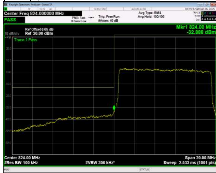
Band26(824-849) QPSK BW=10MHz Channel=26990 RB Size=1 Position=#0 Normal
