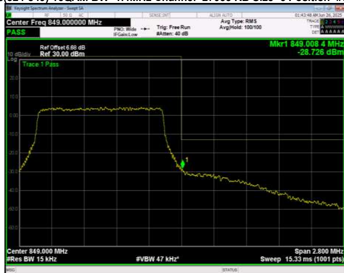
Band26(824-849) 16QAM BW=10MHz Channel=26840 RB Size=1 Position=#0 Normal
