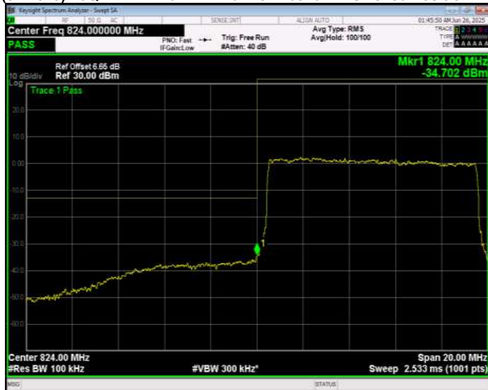
Band26(824-849) 16QAM BW=10MHz Channel=26990 RB Size=1 Position=#0 Normal
