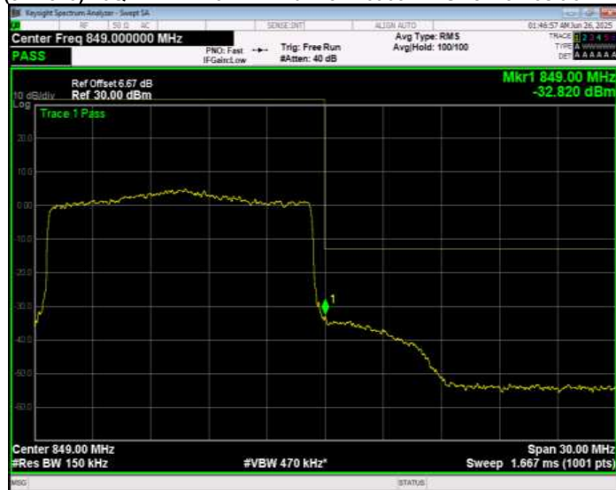
Band26(824-849) 16QAM BW=3MHz Channel=26805 RB Size=1 Position=#0 Normal
