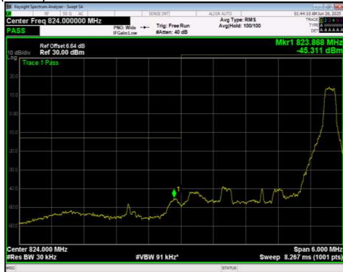
Band26(824-849) 16QAM BW=3MHz Channel=26805 RB Size=15 Position=#0 Normal
