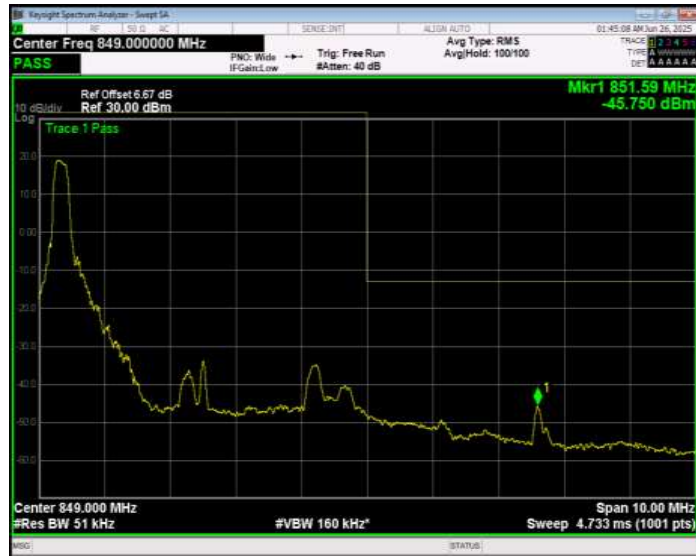
Band26(824-849) QPSK BW=5MHz Channel=27015 RB Size=1 Position=#Max Normal
