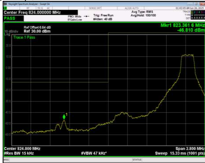
Band26(824-849) QPSK BW=1.4MHz Channel=26797 RB Size=6 Position=#0 Normal
