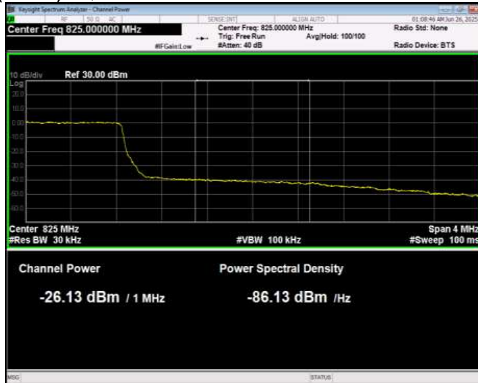
Band26(814-824) 16QAM BW=3MHz Channel=26775 RB Size=15 Position=#0 Normal
