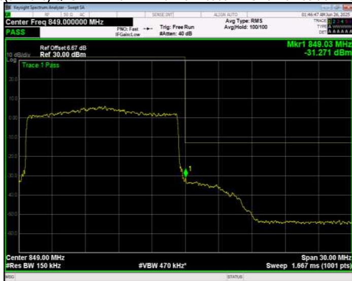
Band26(824-849) QPSK BW=3MHz Channel=26805 RB Size=1 Position=#0 Normal
