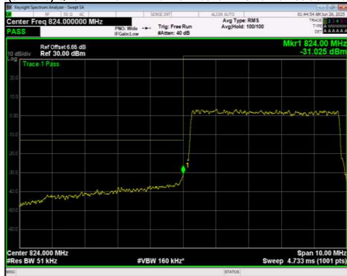
Band26(824-849) QPSK BW=5MHz Channel=27015 RB Size=1 Position=#0 Normal
