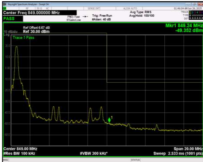
Band26(824-849) 16QAM BW=10MHz Channel=26990 RB Size=1 Position=#Max Normal
