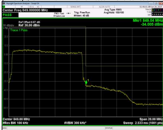
Band26(824-849) QPSK BW=15MHz Channel=26865 RB Size=1 Position=#0 Normal
