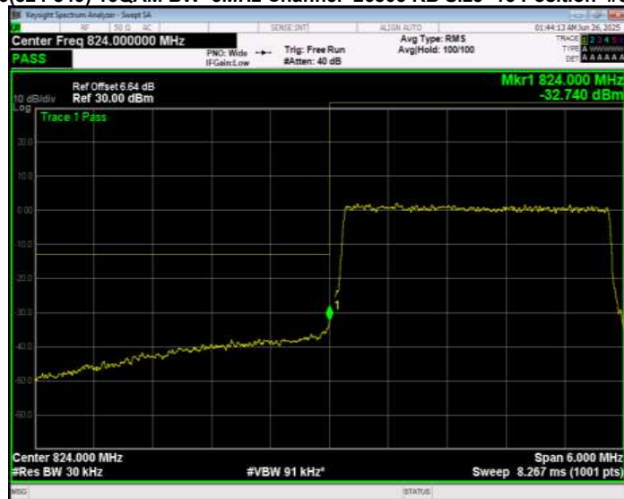
Band26(824-849) 16QAM BW=3MHz Channel=27025 RB Size=1 Position=#0 Normal
