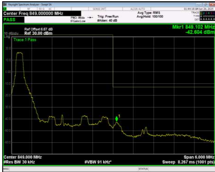
Band26(824-849) QPSK BW=3MHz Channel=27025 RB Size=1 Position=#Max Normal
