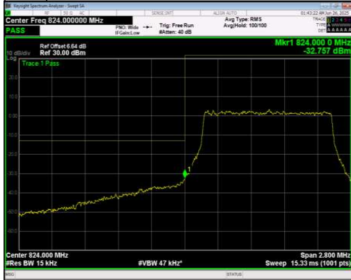
Band26(824-849) 16QAM BW=1.4MHz Channel=27033 RB Size=1 Position=#0 Normal
