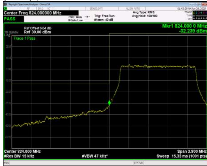
Band26(824-849) QPSK BW=1.4MHz Channel=27033 RB Size=1 Position=#0 Normal
