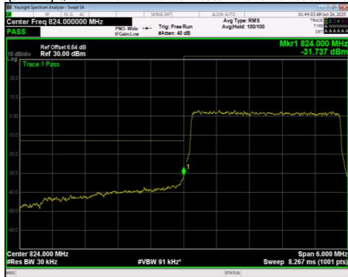
Band26(824-849) QPSK BW=3MHz Channel=27025 RB Size=1 Position=#0 Normal
