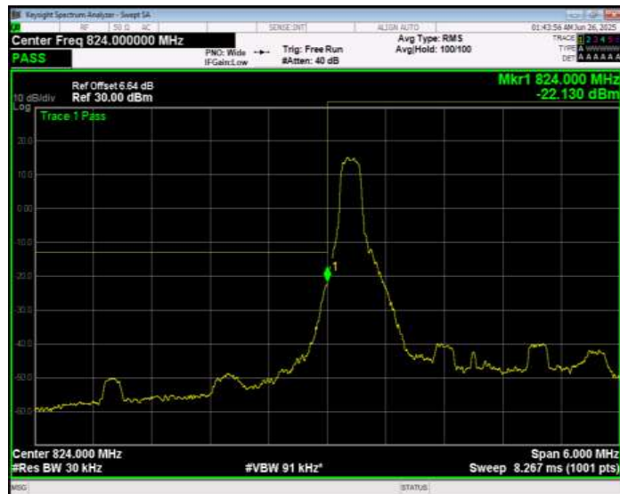
Band26(824-849) QPSK BW=3MHz Channel=26805 RB Size=1 Position=#Max Normal
