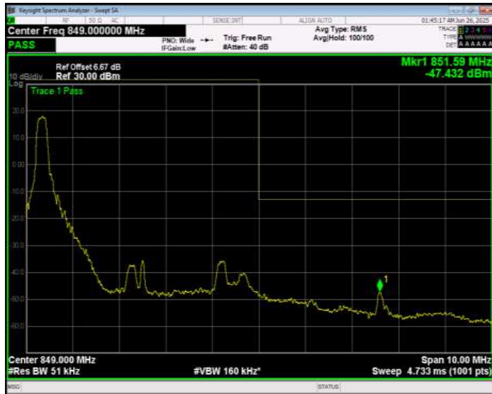
Band26(824-849) 16QAM BW=5MHz Channel=27015 RB Size=1 Position=#Max Normal
