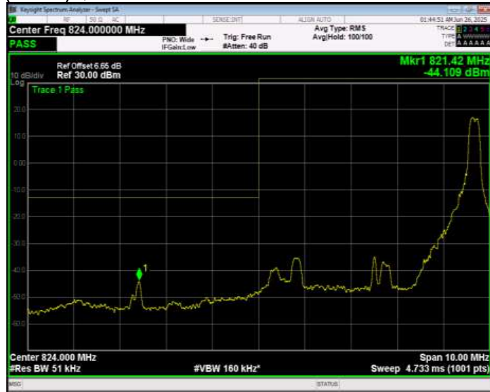
Band26(824-849) QPSK BW=5MHz Channel=26815 RB Size=25 Position=#0 Normal
