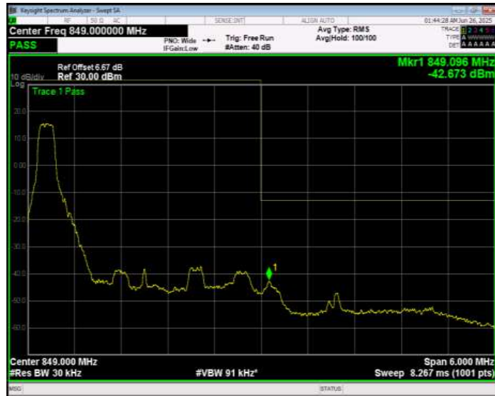
Band26(824-849) 16QAM BW=3MHz Channel=27025 RB Size=1 Position=#Max Normal
