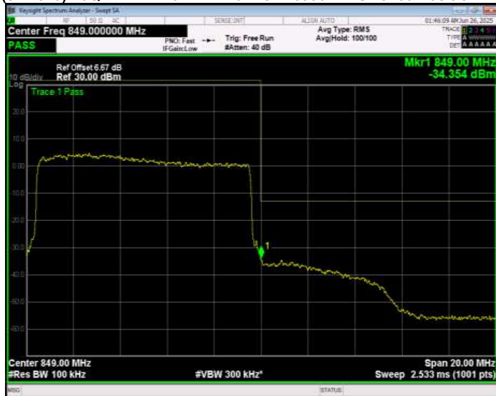
Band26(824-849) 16QAM BW=15MHz Channel=26865 RB Size=1 Position=#0 Normal
