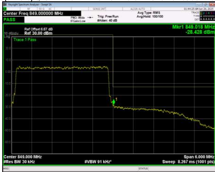
Band26(824-849) QPSK BW=5MHz Channel=26815 RB Size=1 Position=#0 Normal
