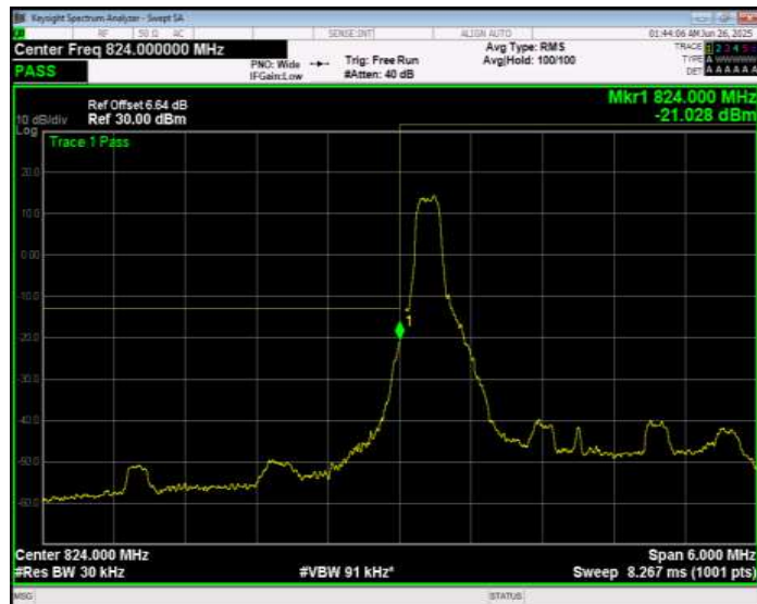
Band26(824-849) 16QAM BW=3MHz Channel=26805 RB Size=1 Position=#Max Normal
