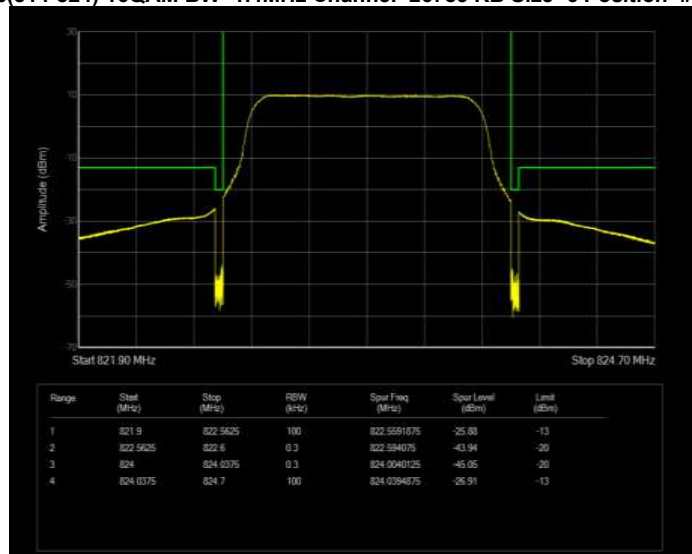
Band26(814-824) 16QAM BW=10MHz Channel=26740 RB Size=1 Position=#0 Extended
