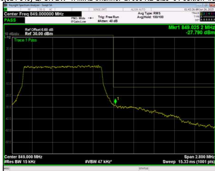
Band26(824-849) QPSK BW=10MHz Channel=26840 RB Size=1 Position=#0 Normal
