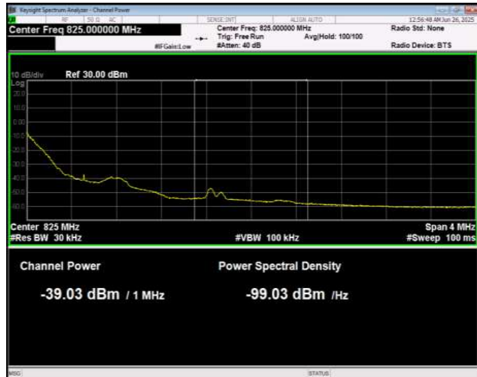
Band26(814-824) 16QAM BW=1.4MHz Channel=26783 RB Size=1 Position=#0 Normal
