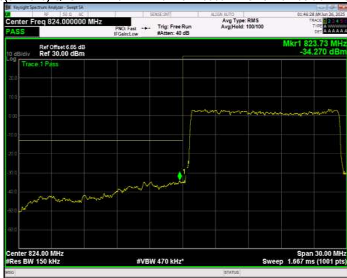
Band26(824-849) QPSK BW=15MHz Channel=26965 RB Size=1 Position=#0 Normal
