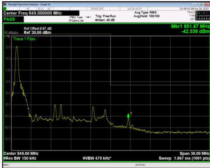
Band26(824-849) QPSK BW=15MHz Channel=26965 RB Size=1 Position=#Max Normal
