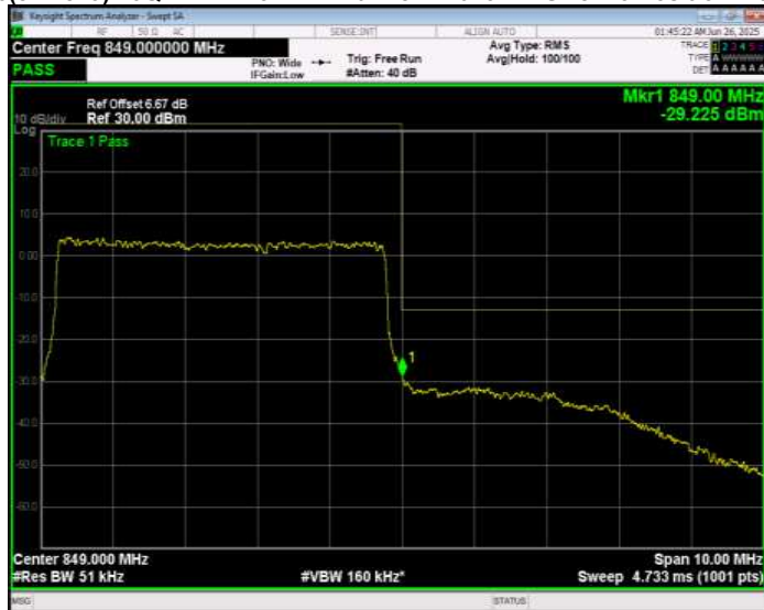
Band26(824-849) QPSK BW=1.4MHz Channel=26797 RB Size=1 Position=#0 Normal
