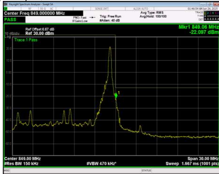
Band26(824-849) 16QAM BW=15MHz Channel=26965 RB Size=75 Position=#0 Normal
