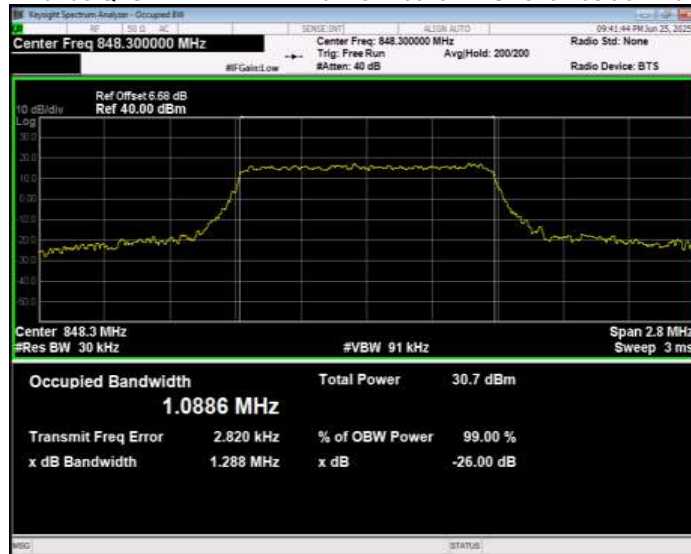
Band5 QPSK BW=10MHz Channel=20450 RB Size=50 Position=#0
