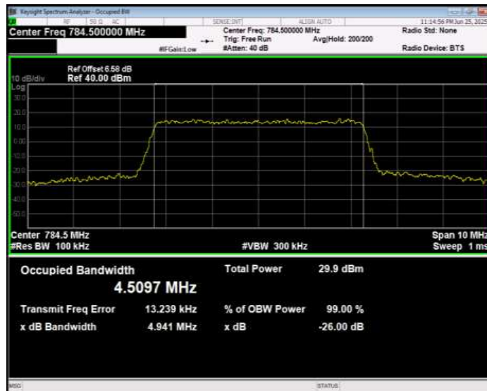
Band13 QPSK BW=10MHz Channel=23230 RB Size=50 Position=#0
