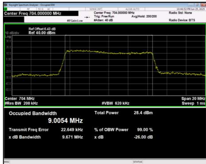
Band12 QPSK BW=10MHz Channel=23095 RB Size=50 Position=#0
