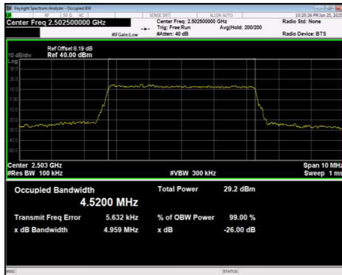
Band7 QPSK BW=5MHz Channel=21100 RB Size=25 Position=#0
