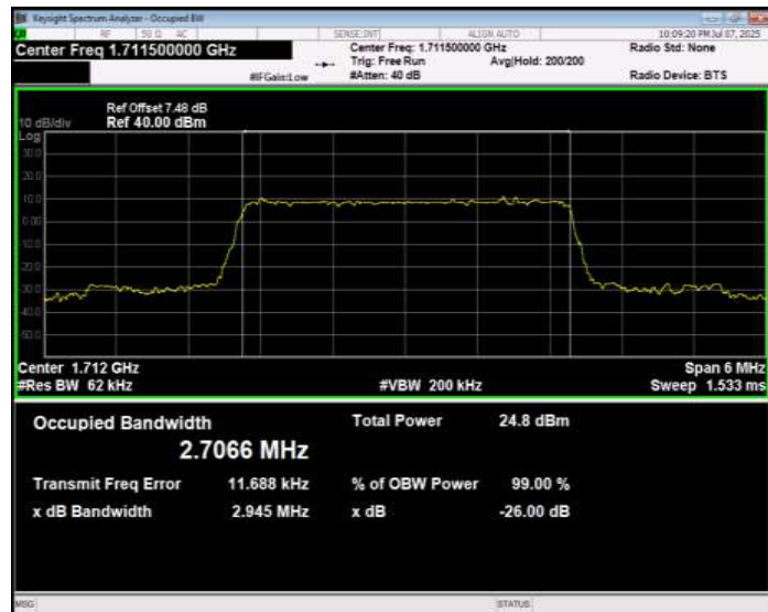
Band4 QPSK BW=3MHz Channel=20175 RB Size=15 Position=#0
