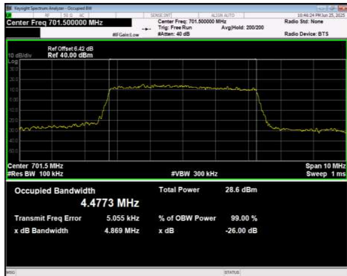
Band12 QPSK BW=5MHz Channel=23095 RB Size=25 Position=#0
