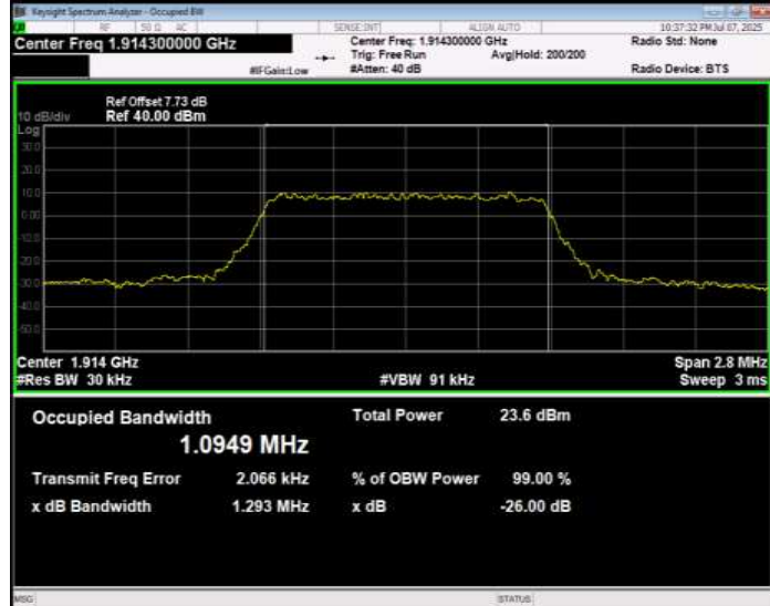
Band25 16QAM BW=10MHz Channel=26090 RB Size=50 Position=#0
