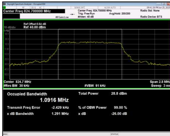
Band5 QPSK BW=1.4MHz Channel=20525 RB Size=6 Position=#0
