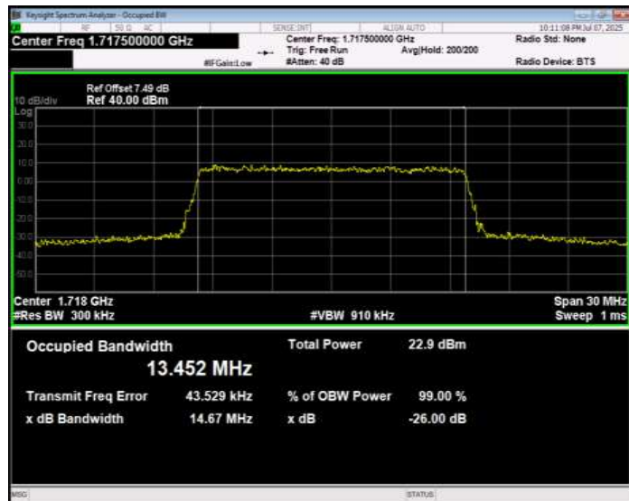
Band4 16QAM BW=15MHz Channel=20175 RB Size=75 Position=#0
