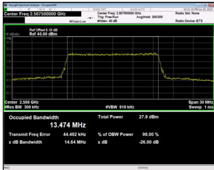
Band7 16QAM BW=15MHz Channel=21100 RB Size=75 Position=#0
