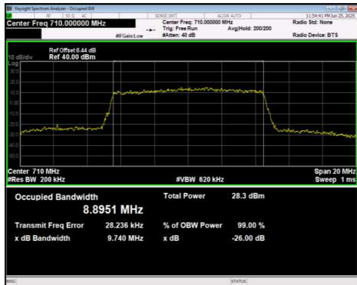
Band17 QPSK BW=10MHz Channel=23800 RB Size=50 Position=#0
