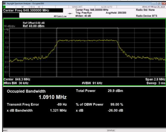
Band5 16QAM BW=10MHz Channel=20450 RB Size=50 Position=#0
