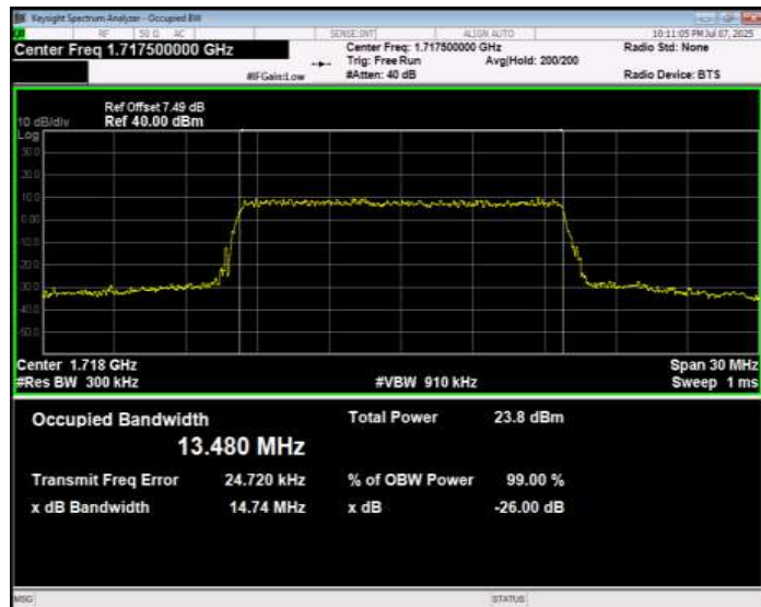
Band4 QPSK BW=15MHz Channel=20175 RB Size=75 Position=#0
