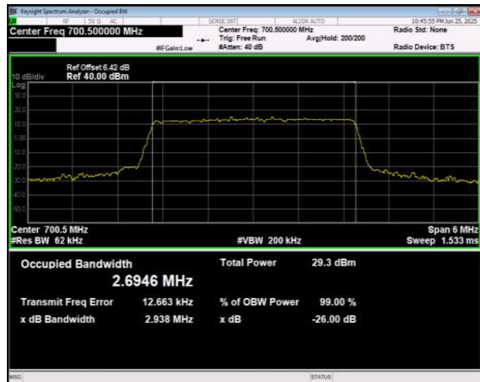
Band12 QPSK BW=3MHz Channel=23095 RB Size=15 Position=#0
