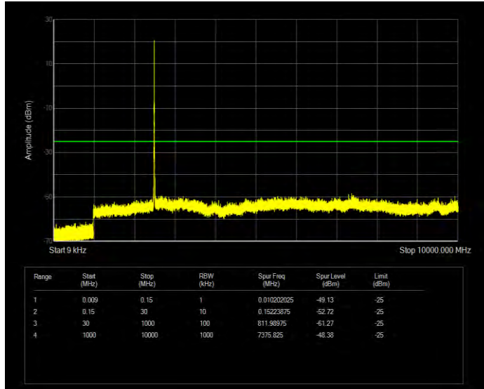
Band7 QPSK BW=5MHz Channel=21100 RB Size=25 Position=#0
