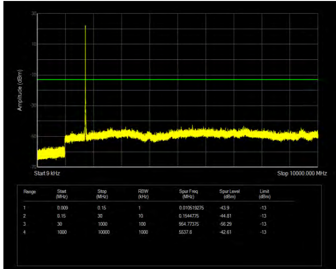
Band4 QAM16 BW=5MHz Channel=20375 RB Size=25 Position=#0
