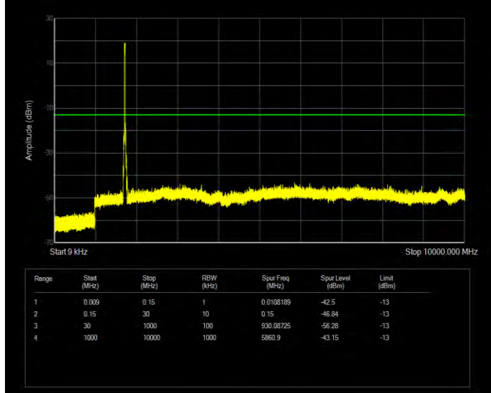
Band4 QPSK BW=20MHz Channel=20300 RB Size=100 Position=#0
