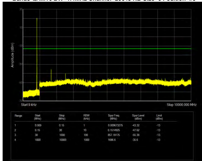
Band5 QAM16 BW=1.4MHz Channel=20643 RB Size=6 Position=#0
