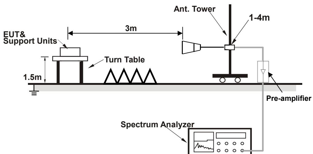
**For radiated test above 18GHz**
