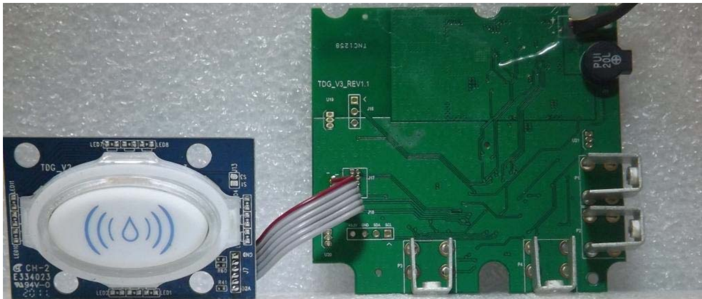
Figure E22.5 – PCB Assemblies Removed
