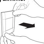
2 Pull the **blue tab** outwards to release the switch
