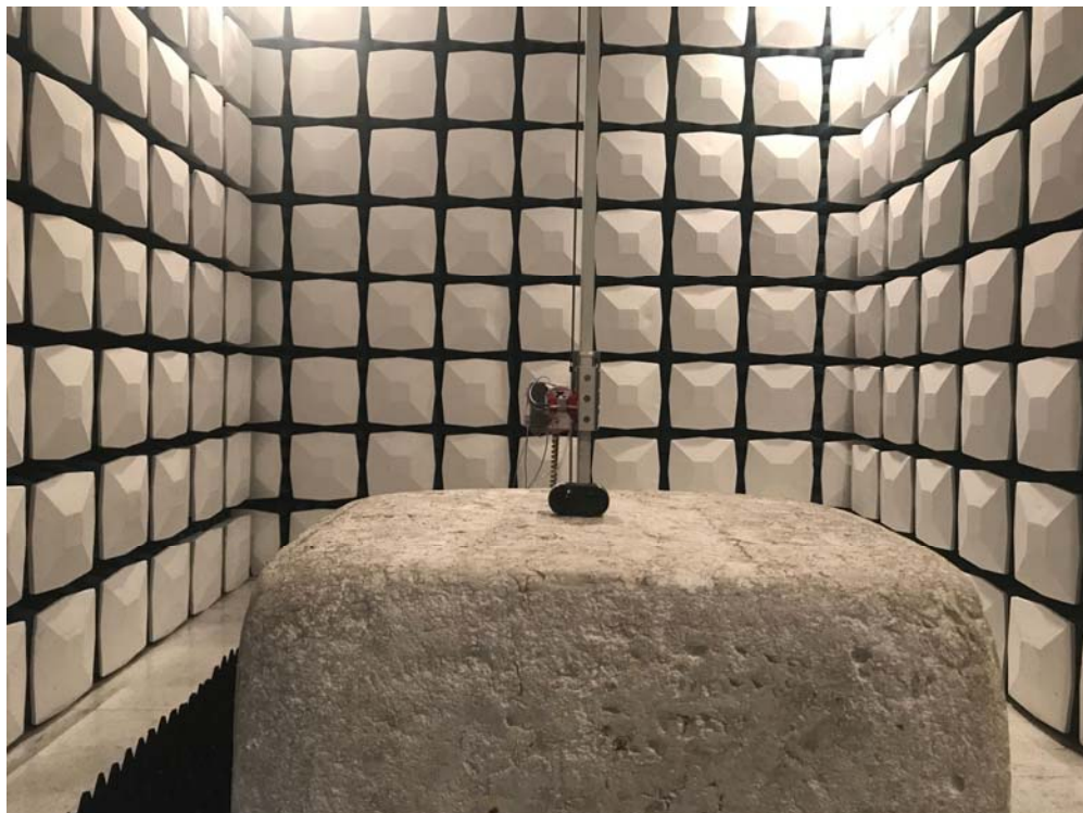
Description: Radiated Emission Test Setup for 1~18GHz
