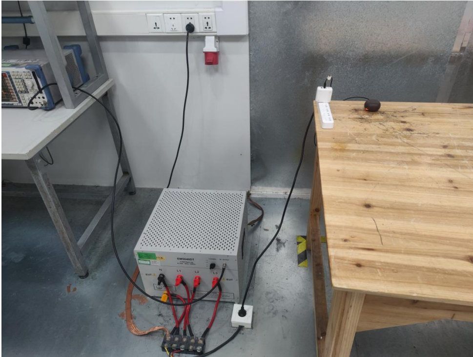
Photo of Conducted Emission Measurement
