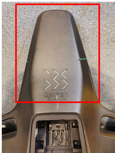
Figure 3. Location of the antennas
