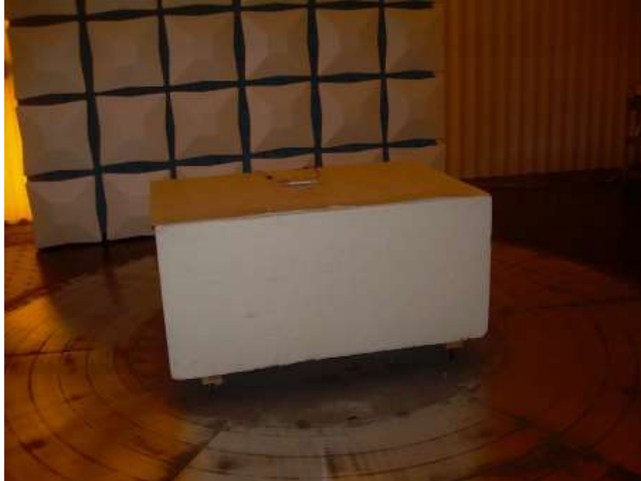
Photograph 1: Front View Radiated Emissions, Worst Case – Below 1000 MHz Configuration
