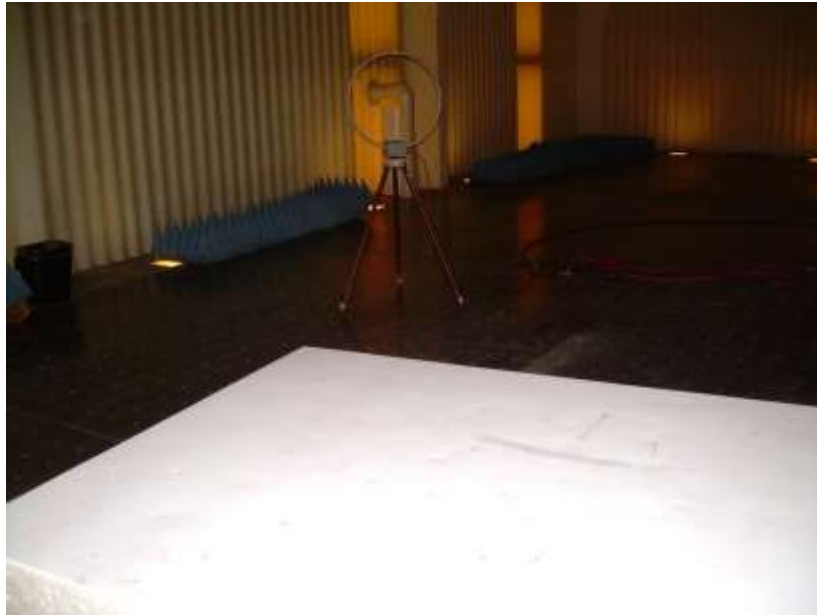
Photograph 6: Reference Photo of Test Setup for Emissions Below 30 MHz
