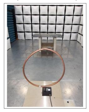
Radiated Spurious Emissions: Less Than 1 GHz
