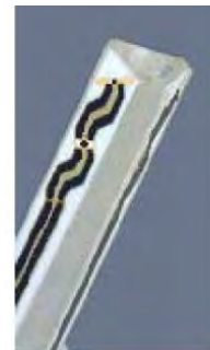
Figure 3.3 Probe Thick-Film Technique
