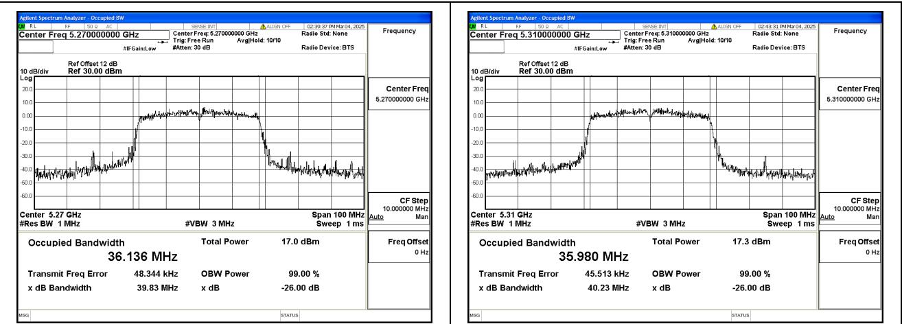
Mode:802.11ac VHT40 Frequency:5270MHz
