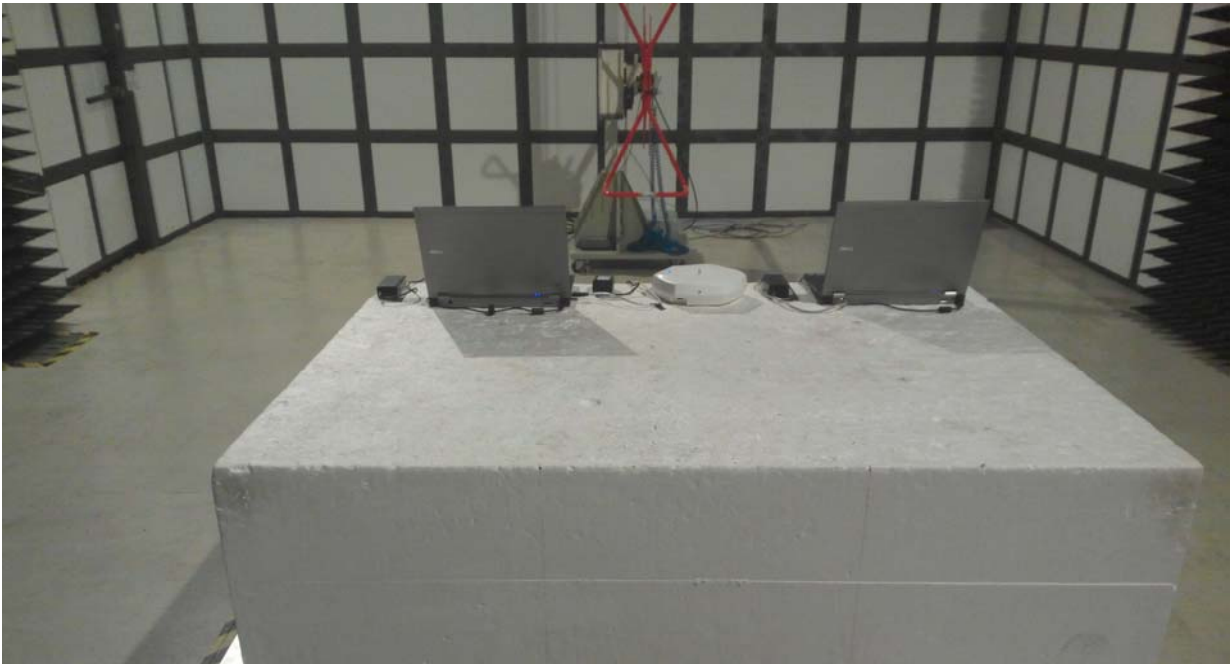
Radiated Emissions- Rear View (Below 1G)
