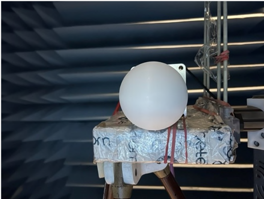
Photograph 2: EUT test setup in ESS_FAC2(>1GHz), EUT elevation 0°_EUT front side_in_respect to measurement
