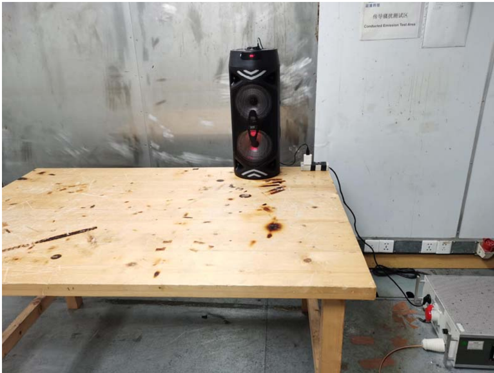
Photo of Radiated Emission Measurement (Below 1G)
