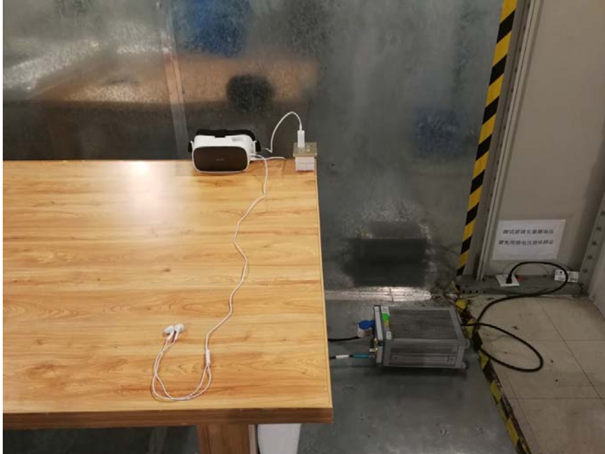
AC power line conducted emissions Side View
