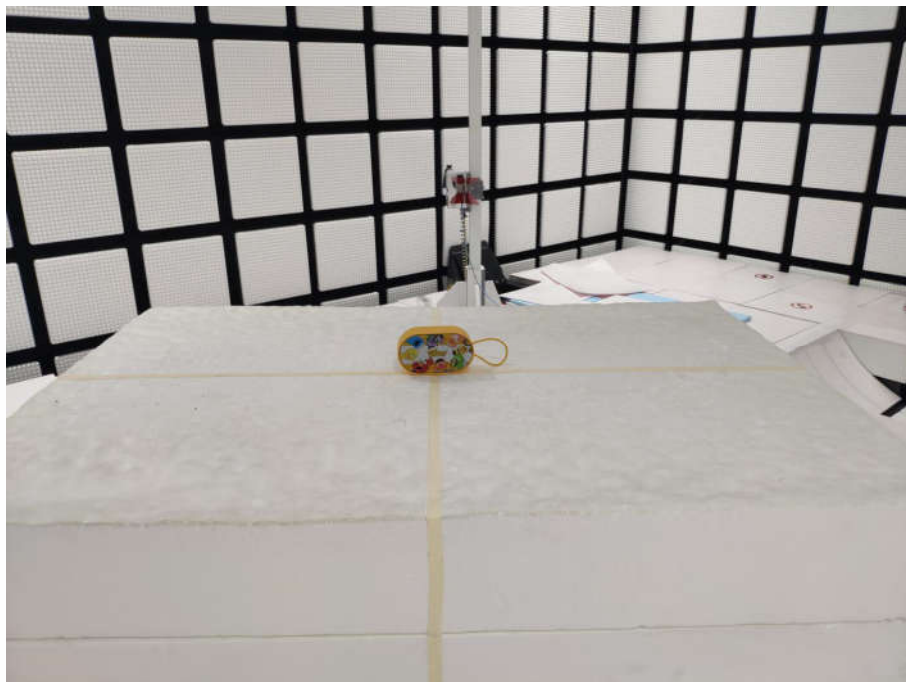
Radiated spurious emission Test Setup-3(Above 1GHz)
