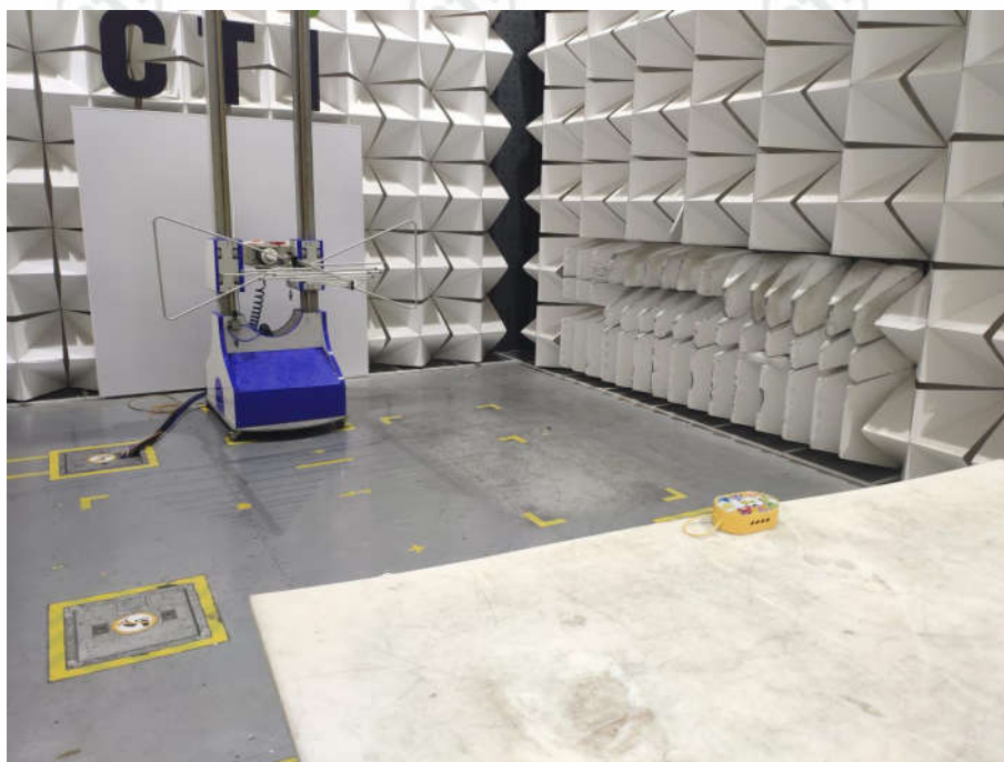
Radiated spurious emission Test Setup-2 (Below 1GHz)
