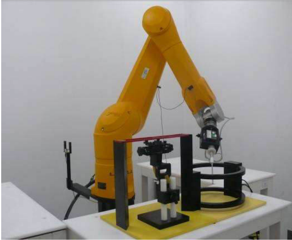
Figure 2 T-Coil Test Measurement Set-up
