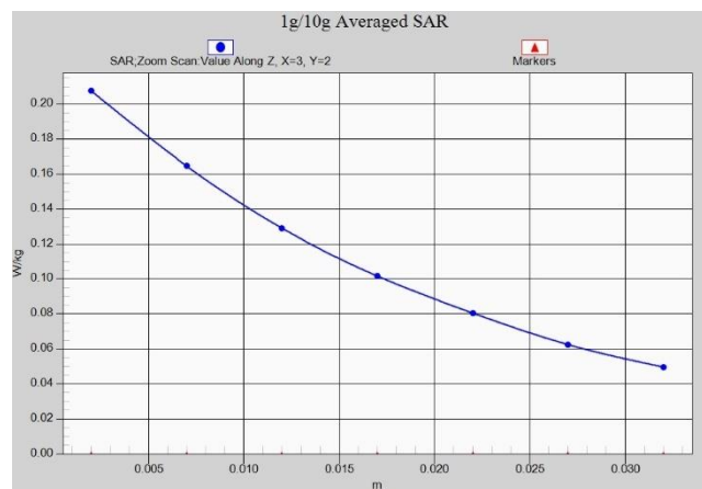
Fig. 1-1 Z-Scan at power reference point (GSM850)
